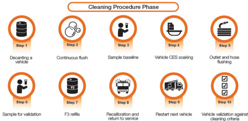
Figure 25: Cleaning procedure phases in accordance to the Queensland DoD (DoD-AUS 2020c)
