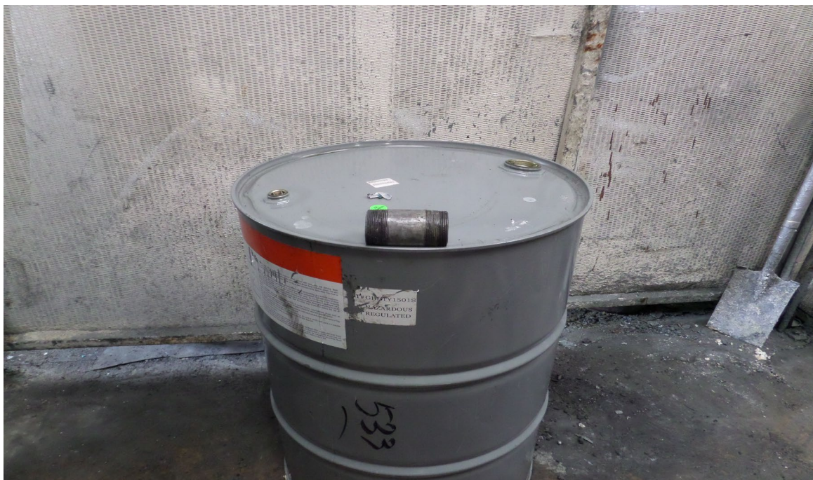
ITW Pro Brands. Chemical Compounding Room. Inspectors observed one 55-gallon container accumulating waste acetone and xylene not kept closed. ITW closed the container. Photograph 4 taken at 11:00 a.m.
