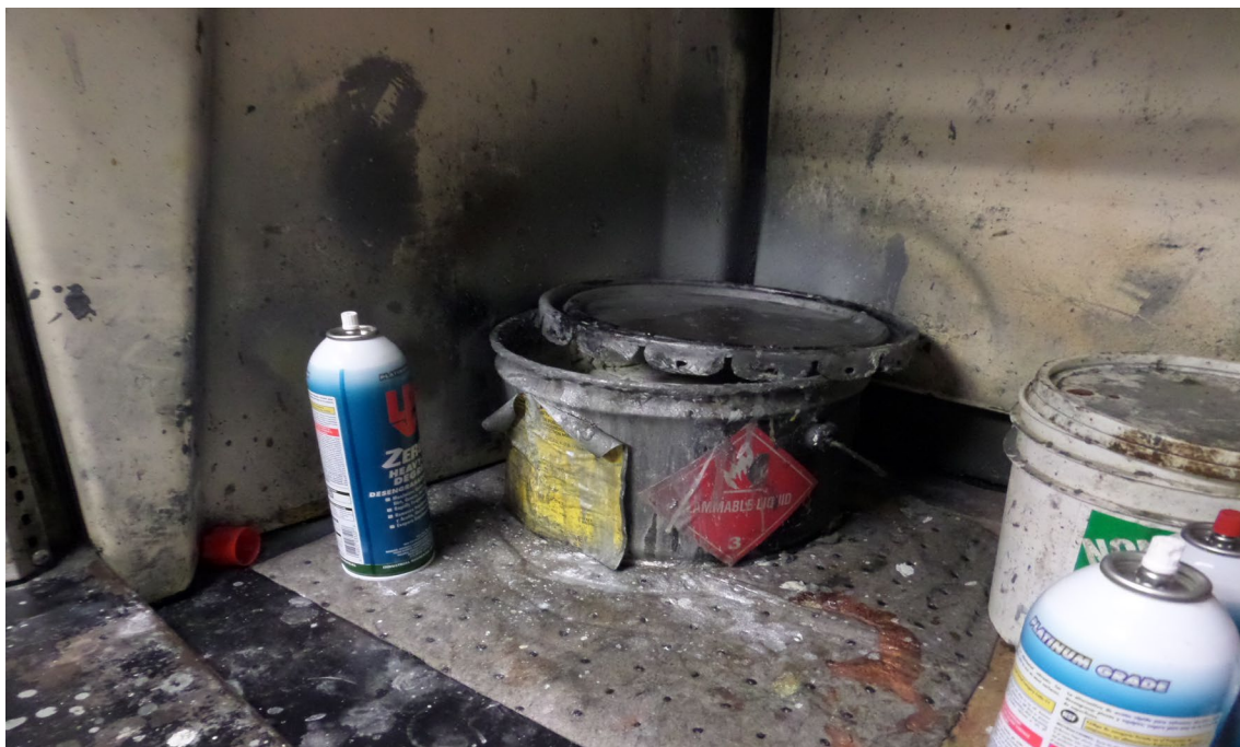
ITW Pro Brands. Quality Assurance Laboratory. Inspectors observed one 2.5-gallon container accumulating waste acetone and xylene inside a fume hood not kept closed. ITW closed the container. Photograph 1 taken at 10:36 a.m.
