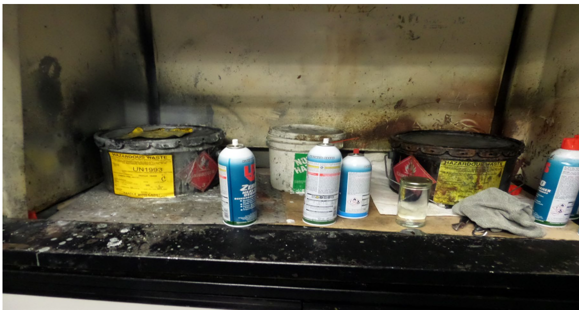
ITW Pro Brands. Quality Assurance Laboratory. Inspectors observed one 2.5-gallon container accumulating waste acetone and xylene inside a fume hood not kept closed. ITW closed the container. Photograph 2 taken at 10:41 a.m.
