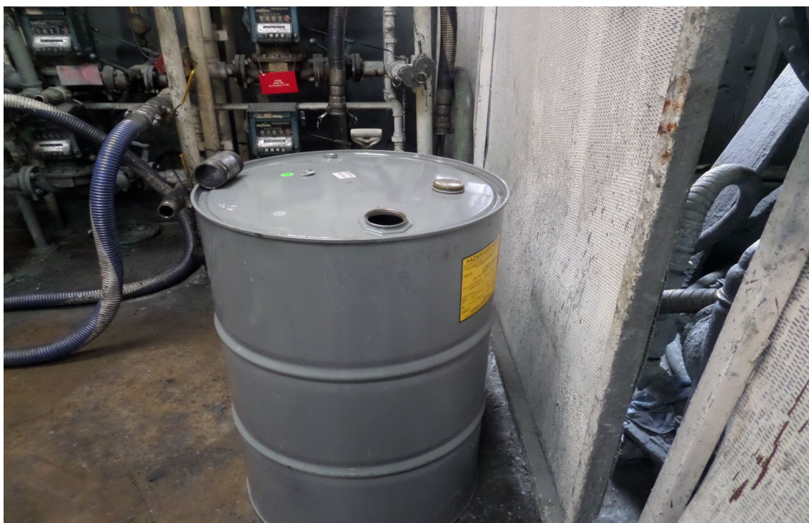
ITW Pro Brands. Chemical Compounding Room. Inspectors observed one 55-gallon container accumulating waste acetone and xylene not kept closed. ITW closed the container. Photograph 3 taken at 10:58 a.m.
