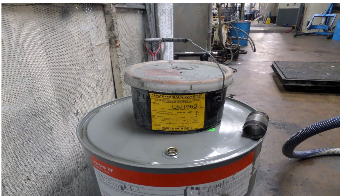
ITW Pro Brands. Chemical Compounding Room. Inspectors observed one 1.5-gallon container accumulating waste acetone and xylene residue not kept closed and not labeled with words hazardous waste. ITW closed and labeled the container. Photograph 6 taken at 11:02 a.m.
