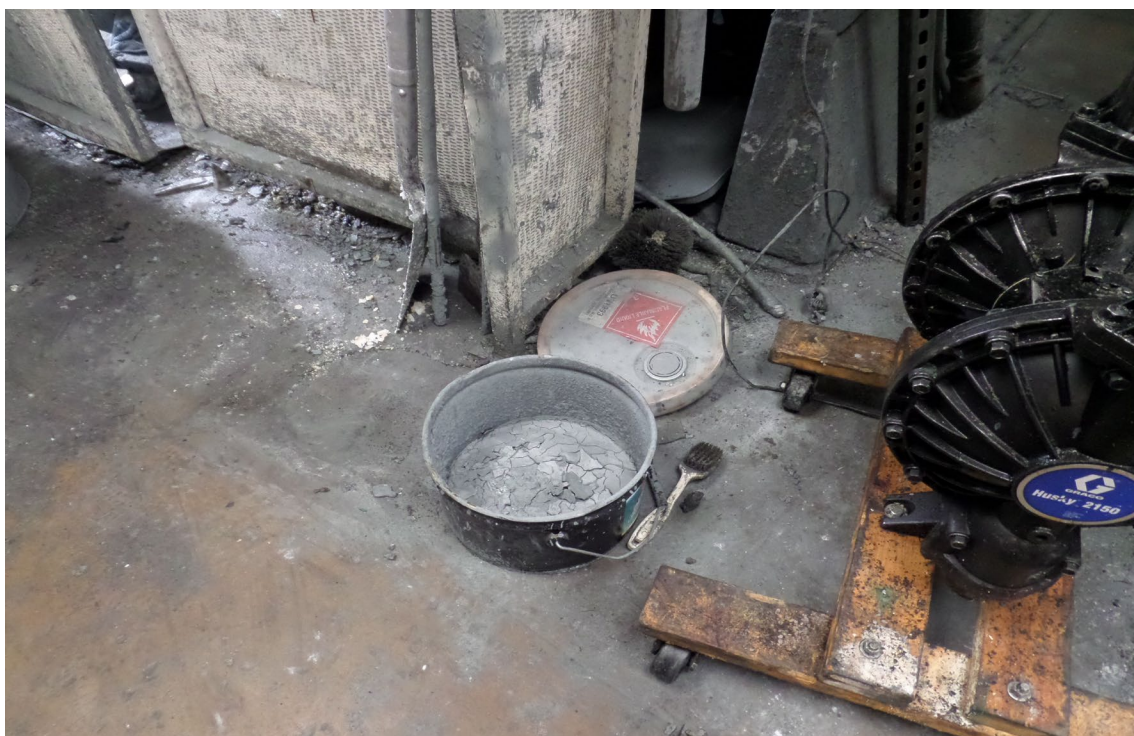
ITW Pro Brands. Chemical Compounding Room. Inspectors observed one 1.5-gallon container accumulating waste acetone and xylene residue not kept closed and not labeled with words hazardous waste. ITW closed and labeled the container. Photograph 5 taken at 11:01 a.m.
