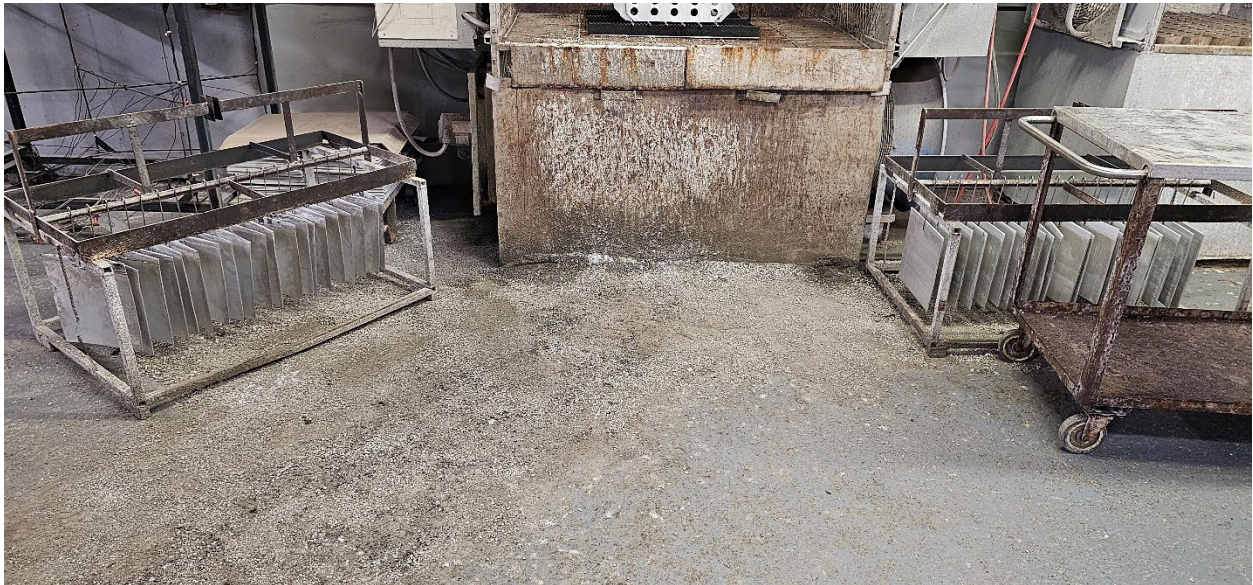
Figure 1: This figure shows the hazardous waste mixed-speedy dry that was observed scattered across the entire dip brazing pot area. The hazardous waste mixed speedy dry material was also observed outside the dip brazing area most likely from foot traffic in this area. The facility representative said there is no sump or collection system in place to collect the hazardous waste and move it to a proper hazardous waste storage container.
