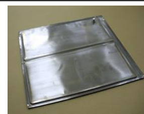
Figure 2.13 Vacuum panel used in domestic appliance
