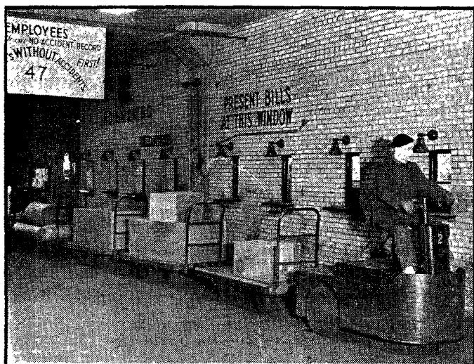
3 Tractor trains haul parcels to outgoing shipping platforms, where they are picked up by . . .
