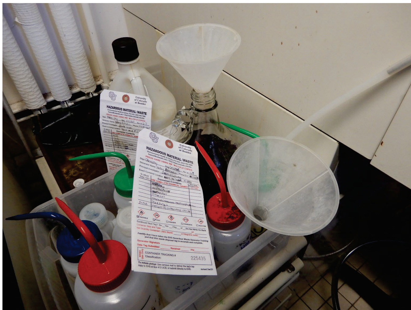
Photo 3 (DSCN0054.JPG): SAA in Cristol Chemistry Rooms 65 and 67 – Luca Research Lab with an open 1-gallon container with a funnel in the top. This container was determined to be in use at the time of the inspection.
