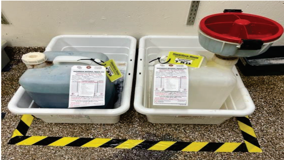
M1B10: Hazardous waste tags attached, caution tape on floor
