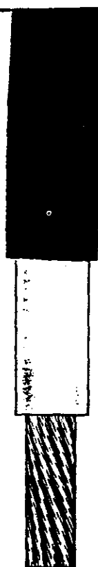
POWER CABLE For voltages of 600 to 5000 volts. With tinned copper, stranded conductor; silicone rubber insulation; and fiberglass or asbestos braided covering.
