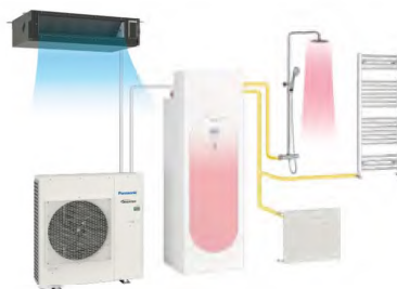
Multi functional split: combination of air-to-air AND air-to-water
