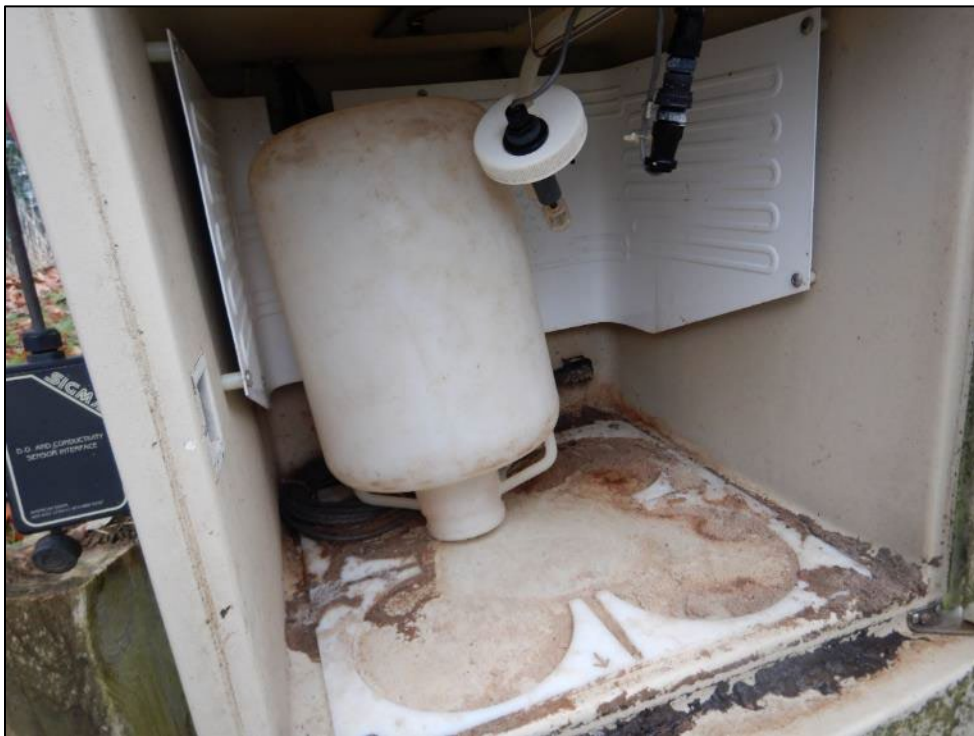
Photograph 26. (DSCN0106). View inside the refrigerator of the automatic composite sampler for Outlet 011. Permittee representatives stated that a calibrated thermometer is not placed inside the refrigerator during sampling. Brown-colored staining was present inside the refrigerator.
