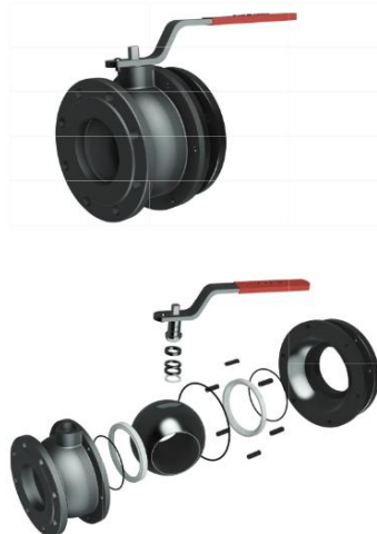
Figure 8: Kalrez® O-ring in ball valves.
