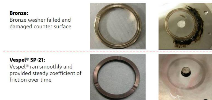
Figure 23: Vespel® thrust washer in comparison to bronze
