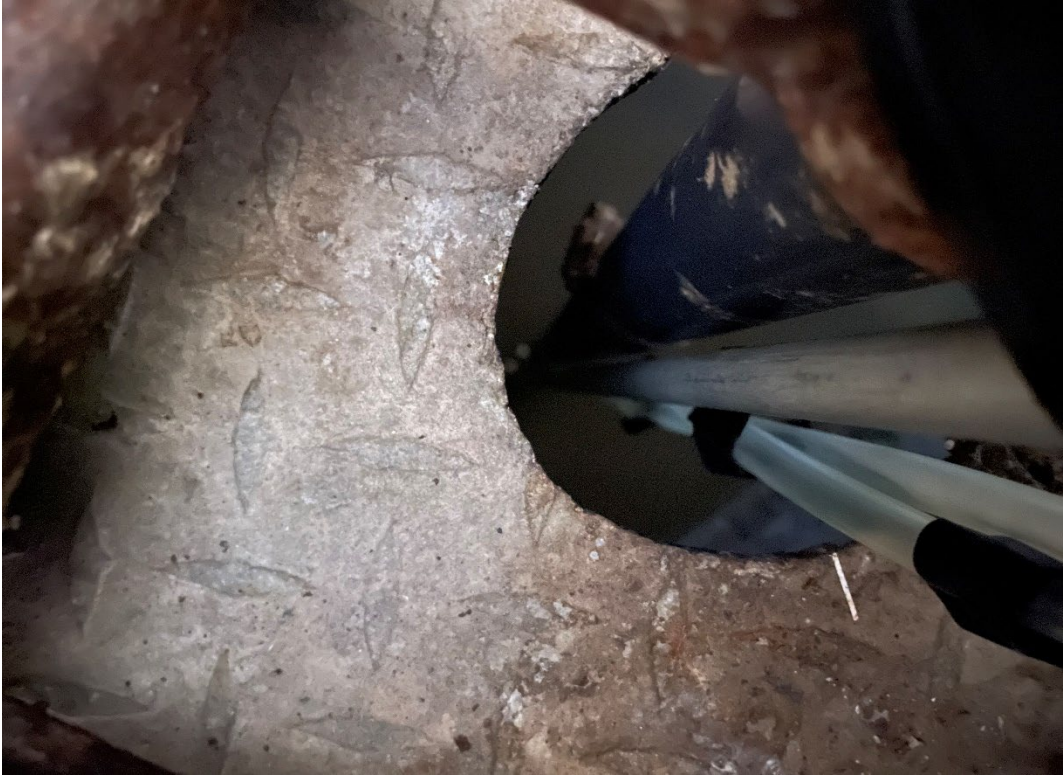
Photo #1. Composite samples were collected before the Parshall Flume.
