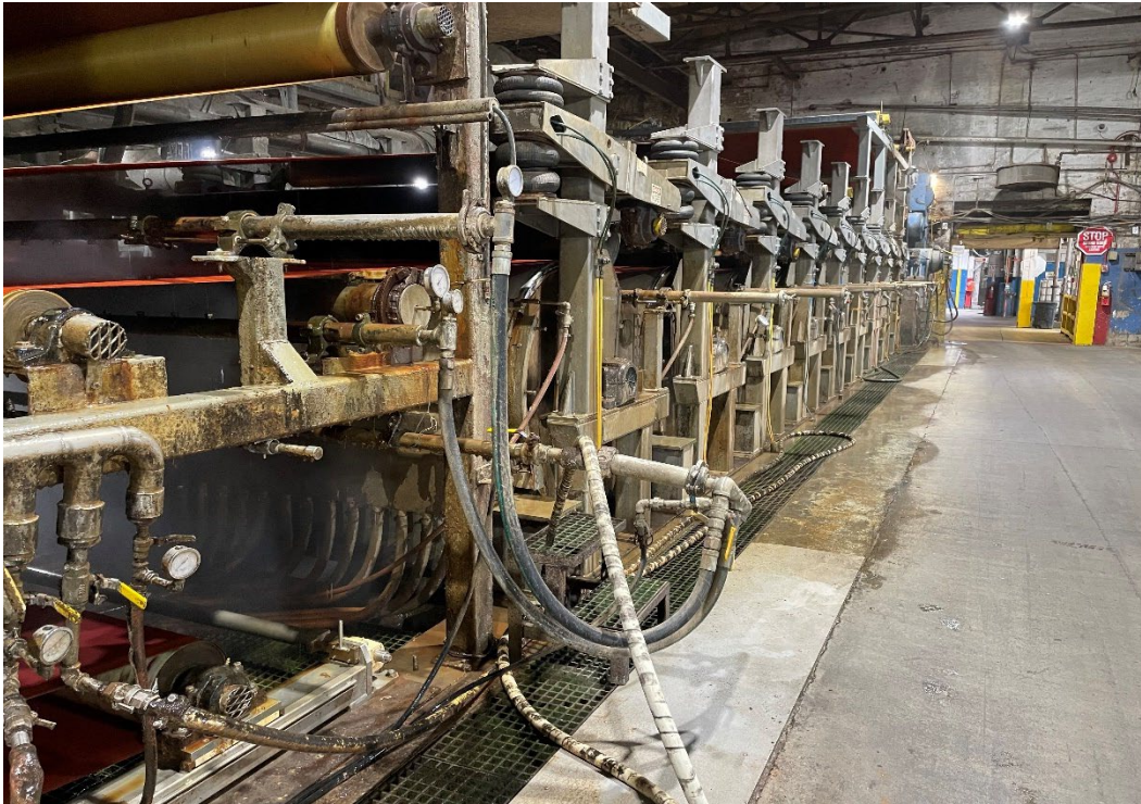
Photo #5. Fine pulp is fed onto the cylinders of the dry paper making machine.
