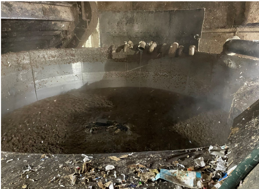
Photo #4. Shredded recycled paper and reclaimed water are used in the pulpers (blender).
