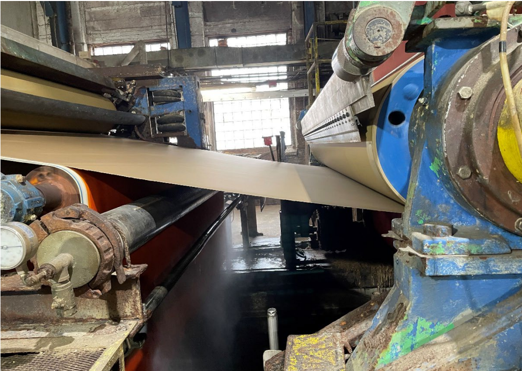
Photo #6. Moisture is driven away from the pulp through the paper making process.
