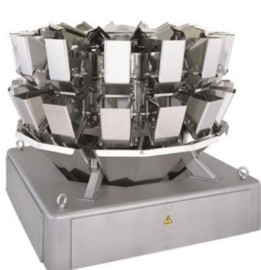
Instrument example (Weigher for food industries)
