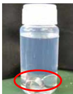
Figure 92 Method for extracting oil from solid samples
