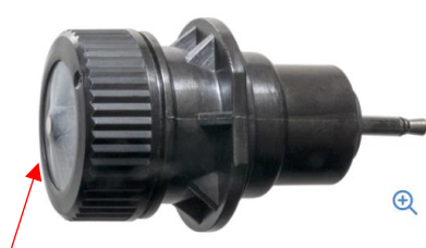
Membrane Dissolved oxygen electrode
