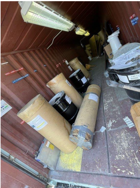
Photograph 29: Connex container for UW. Three UW lamp containers are not fully closed.
