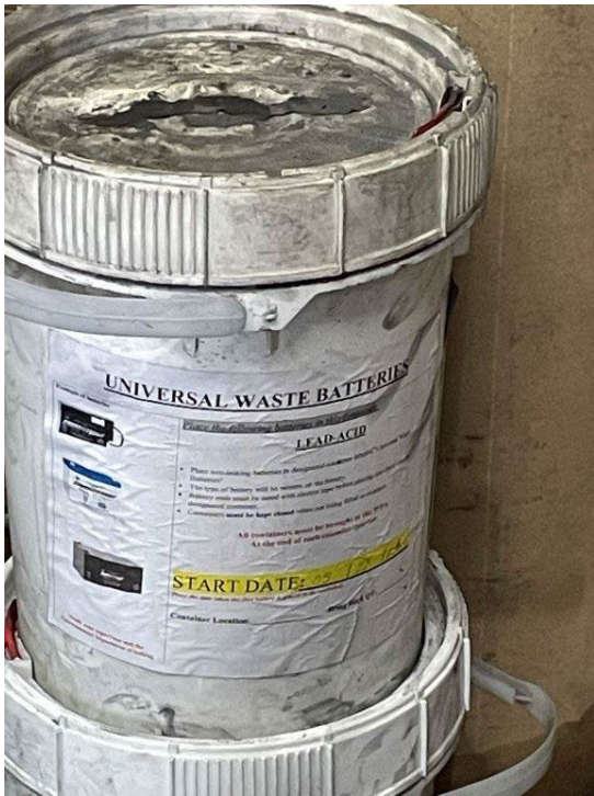
Photograph 9: SA-2A, UW Battery Containers, Containers Labeled and Dated.
