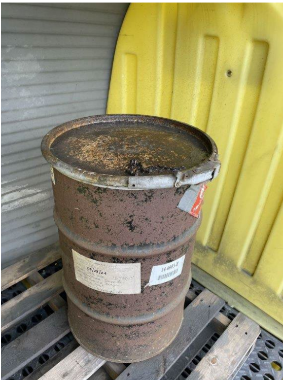
Photograph 26: 30-gallon Metal hazardous waste container that has a significant amount of rusted area.
