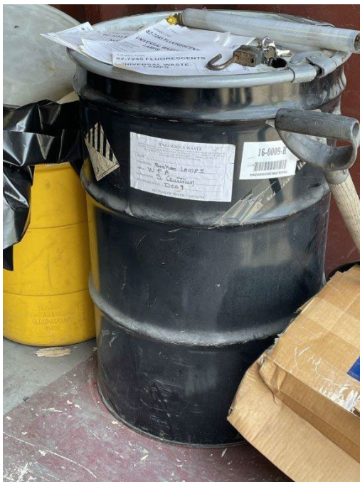
Photograph 28: 55-gallon HW Container of broken lamps that requires a hazard marking.
