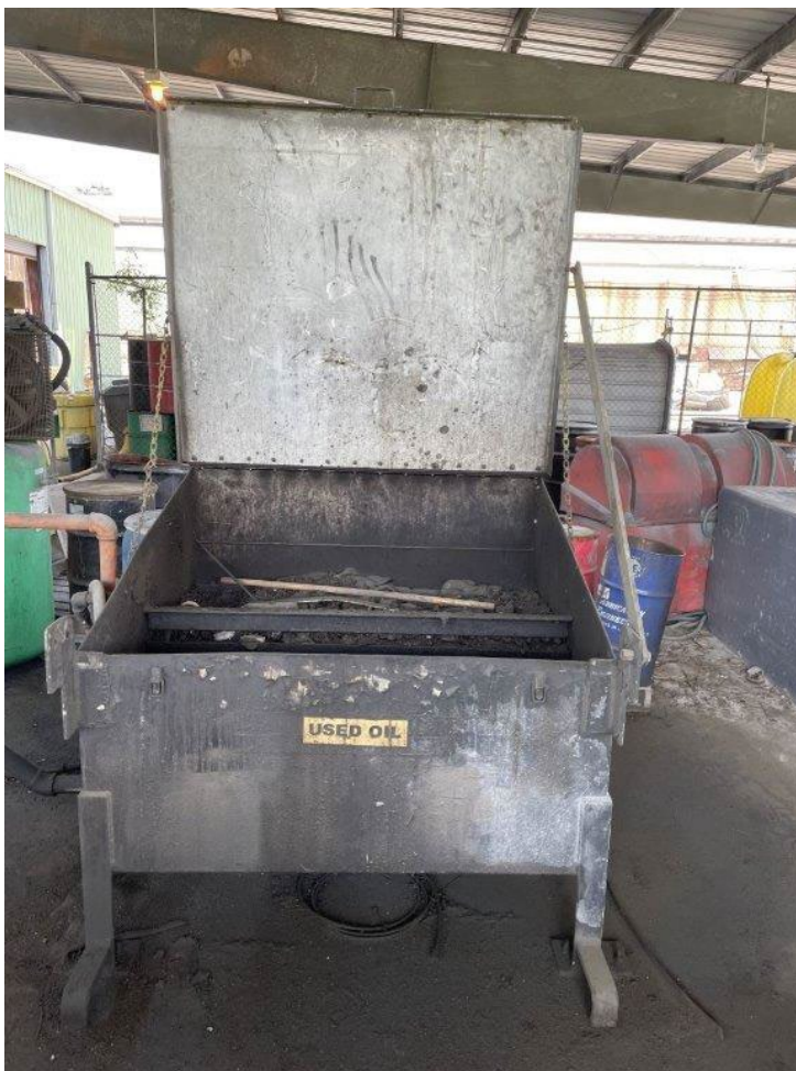
Photograph 19: Used oil draining device.
