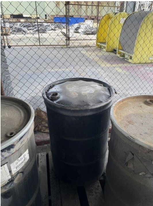
Photograph 25: Oil and grease debris drum that is significantly bulging at the top of the container.
