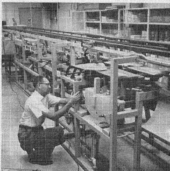
Experimental binder in F&F lab simulates operation of commercial units, is used by customers to solve problems.
