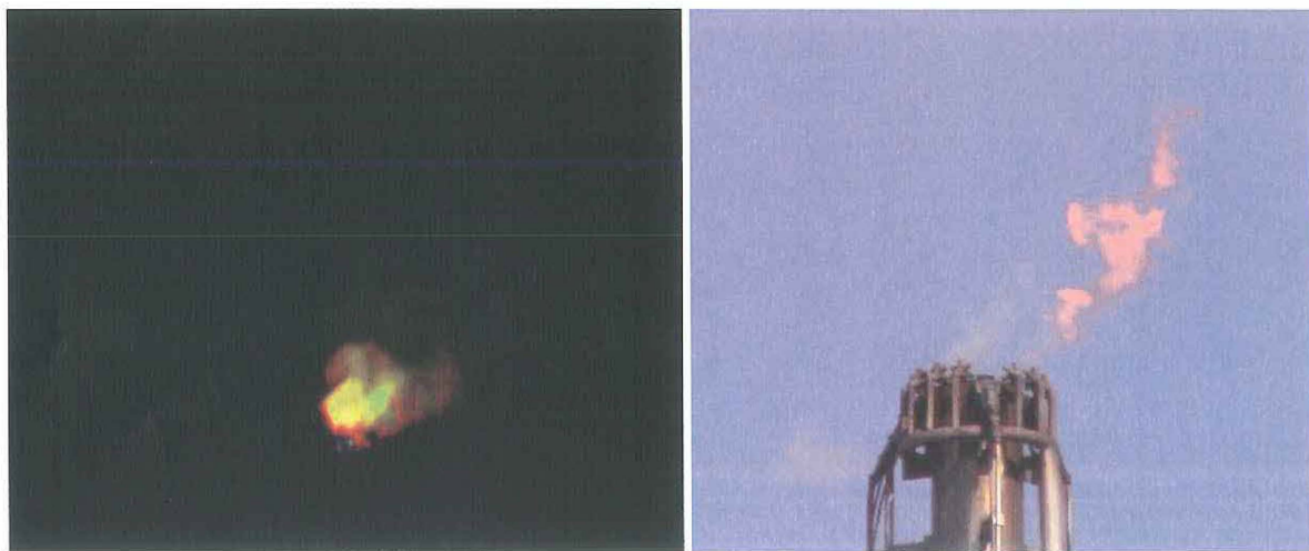
Figure 6. South Flare. Left: A representative composite spectral image generated by VISR instrument. Red color represents \text{CO}_2 ; green color represents hydrocarbon; and blue or bluish white color represents aerosol (e.g., soot) or hot solid object (e.g., the shield for pilots). Right: A representative image in visible spectrum.
