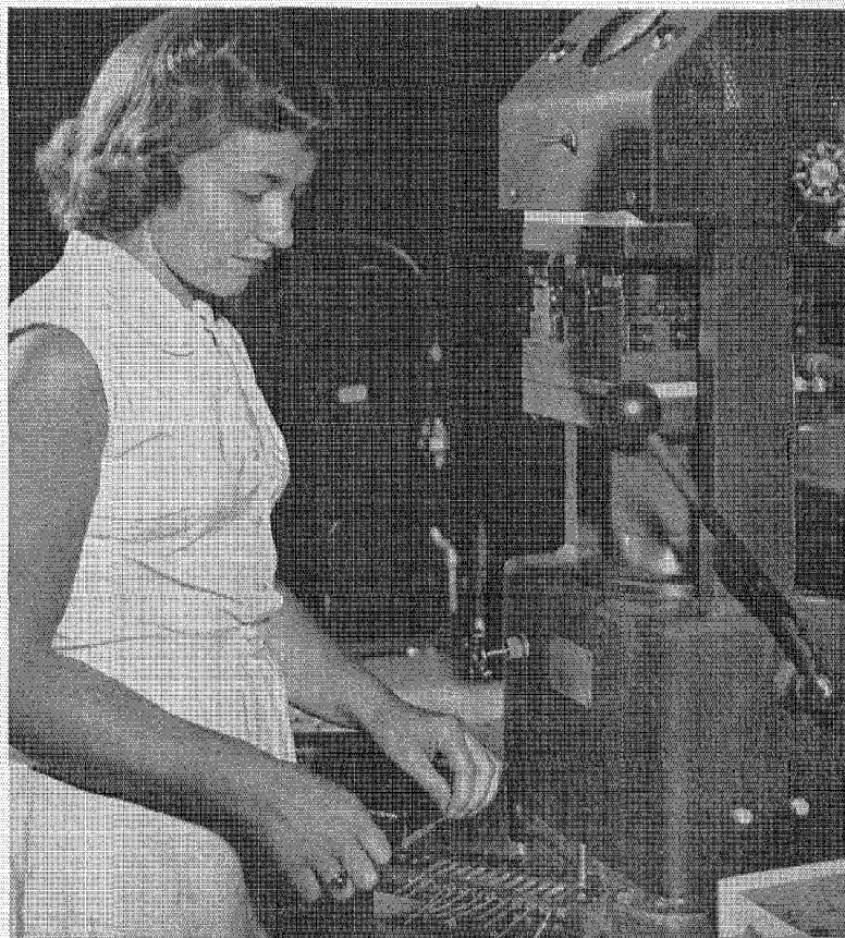
Nylon "envelopes" for thermistors are heat-sealed at Western Electric plant. Ends of tubes are pinched shut in press. In this case, use of nylon has simplified assembly, cut costs.
