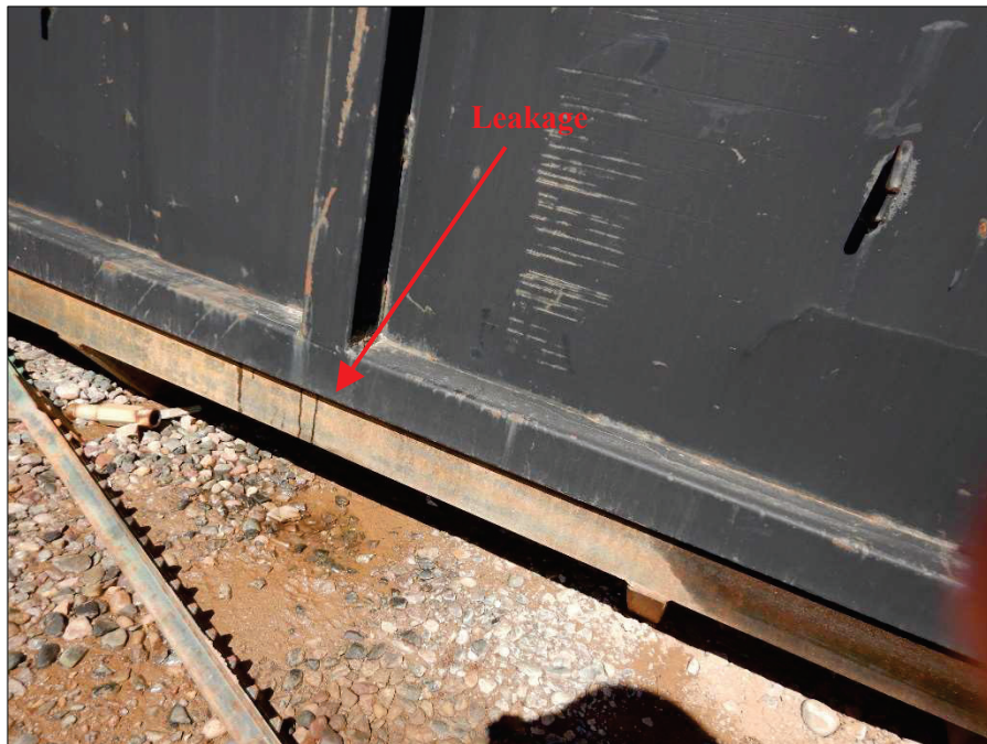
Photograph 37. Additional view of dumpster in boneyard, as referenced in Photographs 35 and 36. Note leakage from dumpster.
