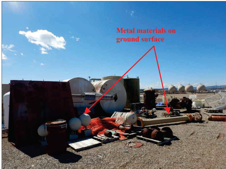
Photograph 32. Additional view, facing Southwest, of the Facility boneyard, as referenced in Photographs 28 through 31. Note materials are uncovered and sitting on the ground. The 55-gallon drum on the left side of the photo was empty at the time of the inspection.
