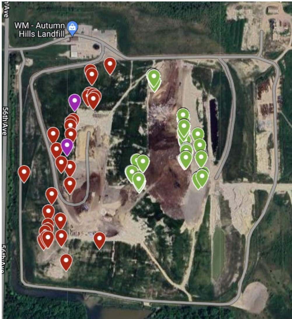
Map of EPA and EGLE SEM Exceedances and Leaking Marker Pipes
