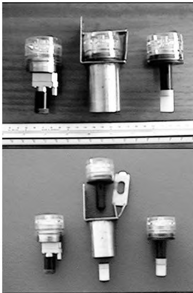
Figure 3: Pictorial view of the BGI stainless steel sampler (left), the cowl sampler (centre) and the without-cowl sampler (right)
