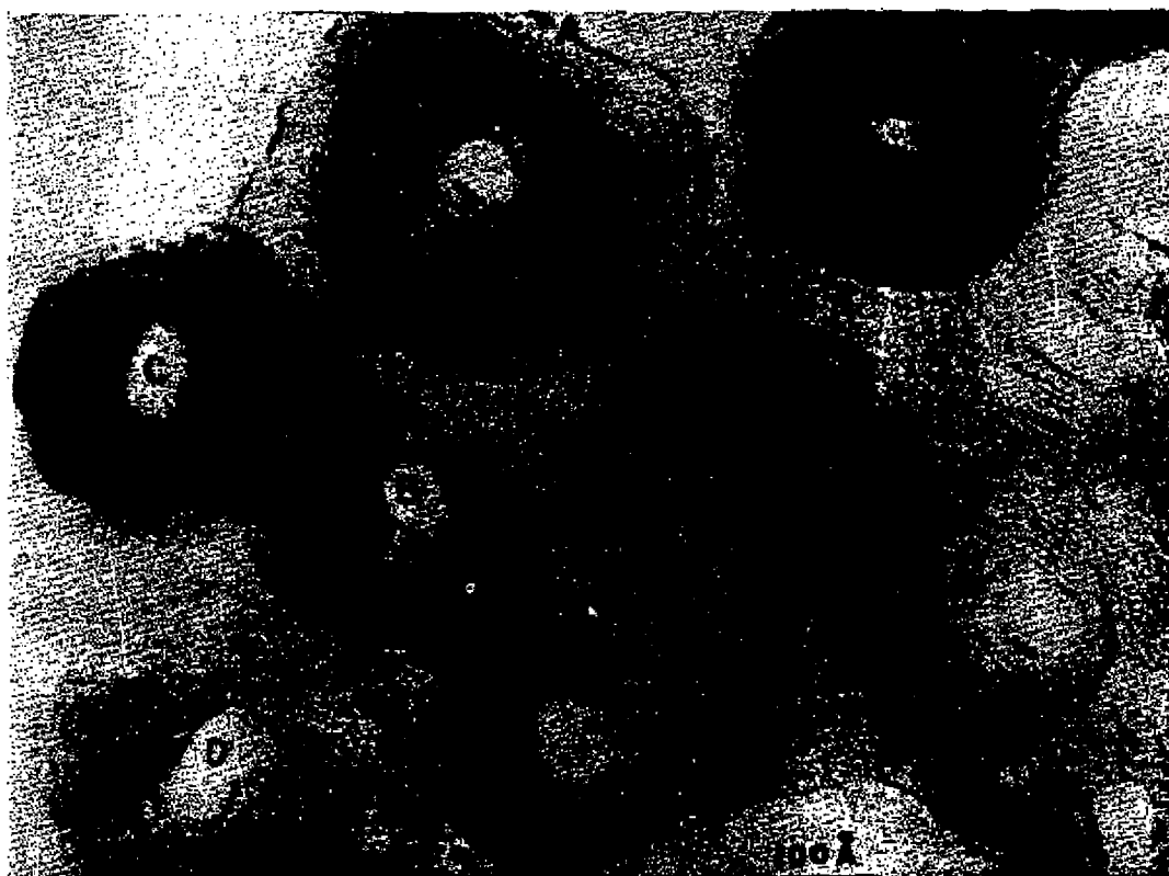
FIG. 3. High resolution transmission electron micrograph of chrysotile fibrils showing its rolled, spiral, structure. The axis of the fibre bundle is perpendicular to the section plane. Fibrils marked as A, B, display round capillaries compared to fibrils C, D, which show oblong capillaries. Fibril F displays a virtually closed capillary. Fibrils range in diameter from \sim 250 Å (C) to \sim 375 Å (A). Note some non-crystalline material in the interfibril area (noted as NC). Fibril packing is not hexagonal as indicated by B fibril which is surrounded by five other fibrils; F fibril which is surrounded by seven other fibrils. Scale marked at the bottom of the plate is 100 Å. Micrograph is from YADA (1967).
