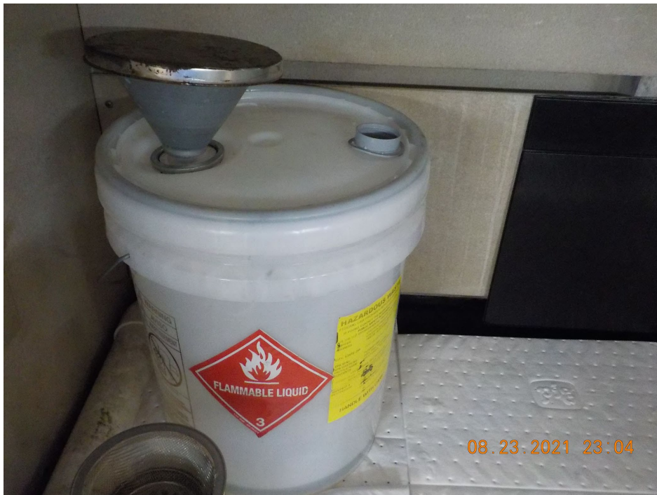
Photo #2 – An open 5-gallon satellite container of hazardous waste in the Test Room.
