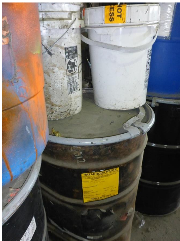
Photo 1: 55-gallon drum in SA-6. The drum, which was labeled D001 hazardous waste aerosol can cylinders and marked with an accumulation start date of 04/11/2021, had a small hole in the lid.
