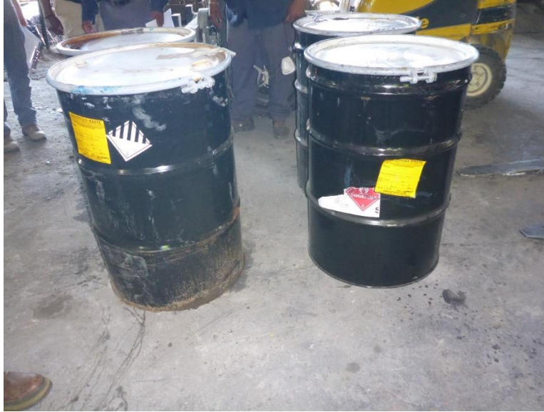
Photo 7: Four 55-gallon drums of F005 / F003 / F004 / F001 / F002 / D001 / D006 / D005 hazardous waste solid (xylene / toluene) in SA-5. Each of the containers was identified with a Class 9 DOT hazard placard. One drum had a portion of a flammable hazard placard, which was part of a previous product label which had been torn off, but none of the containers were clearly identified with an indication that the contents are flammable or toxic.
