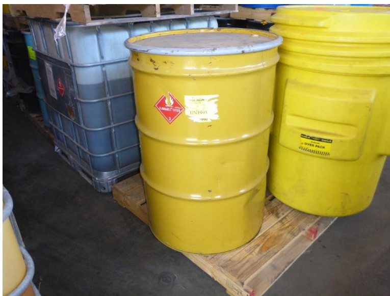
Photo 5: Drum in SA-6 with the hazardous waste label scratched off.
