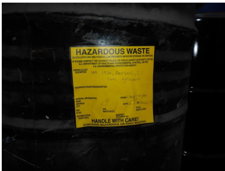
Photo 3: 55-gallon drum in SA-6. Drum labeled hazardous waste flammable aerosol can / cylinder, but not labeled with generator information, EPA waste codes, or an accumulation start date.
