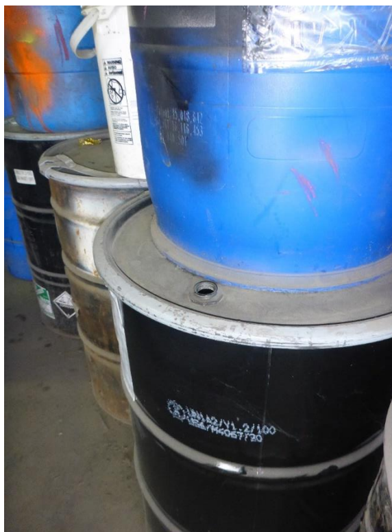
Photo 2: 55-gallon drum in SA-6. The drum, which was labeled as D005 / D006 / D007 / D008 hazardous waste paint filters, was missing a bung.
