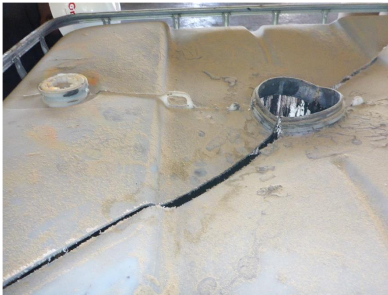
Photo 8: One tote of hazardous waste stacked above other waste containers in SA-5. No hazardous waste label was observed on the tote, which was marked with the tracking number 21-2-16-30. The top of the tote had been cut, leaving the container open and in poor condition. The container label, which had fallen inside the tote, indicated that the tote contained D001 / D035 / F003 / F005 hazardous waste flammable liquid (toluene / MEK).
