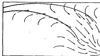
FIG. 6. ELEVATION VIEW OF IMPROPERLY LOCATED RETURN OUTLET
