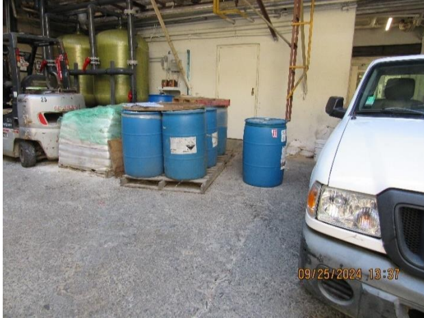
IMG 1379 -Calcium carbonate and other chemicals improperly stored and unprotected from potential damage by operated vehicles in the LUB of Facility.
