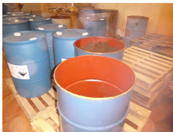
Photograph 17: WWT Filter cake containers
