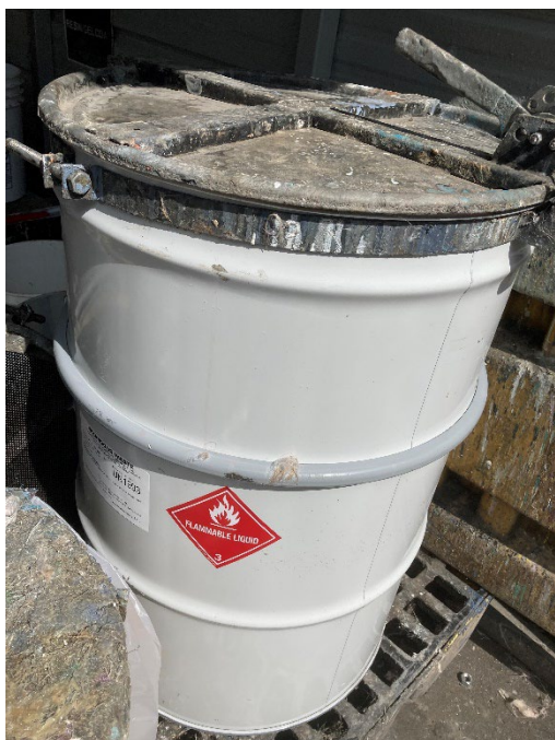
Photo 1, SAA container for spent Thermaclean, Kick-off Shed
