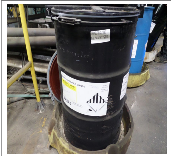
Hager. Oxidizing Line. Inspectors observed a DOT Class 9 (miscellaneous hazardous materials) pictogram on the 55-gallon SAA container. The inspectors observed the container appeared not labeled or marked with an indication of the hazard of the contents. Photograph 9 taken at 10:45 a.m.
