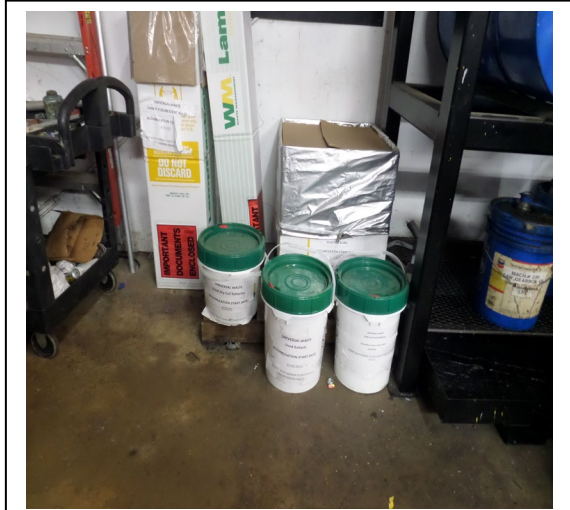
Hager. Maintenance Shop. Inspectors observed several containers accumulating spent lamps and spent batteries. Managed as universal waste. Photograph 4 taken at 10:26 a.m.
