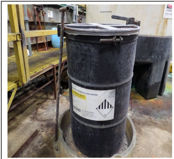
Hager. Plating Department – Line 505 Inspectors observed a DOT Class 9 (miscellaneous hazardous materials) pictogram on the 55-gallon SAA container. The inspectors observed the container appeared not labeled or marked with an indication of the hazard of the contents. Photograph 6 taken at 10:36 a.m.
