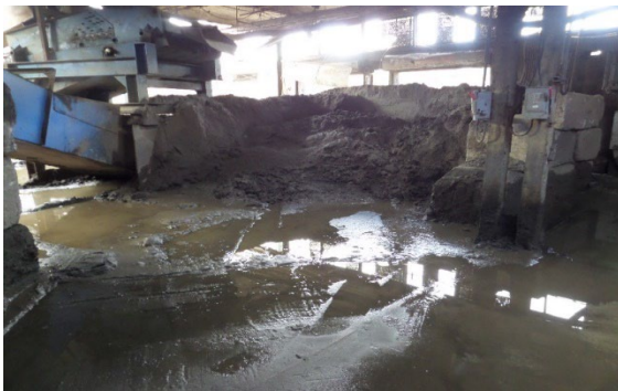
Figure 81: HTL. OKP. Area near to WWT. Observed wastewater, waste solid and sludge behind the filter screen for the spiral line. 4:27 pm.
