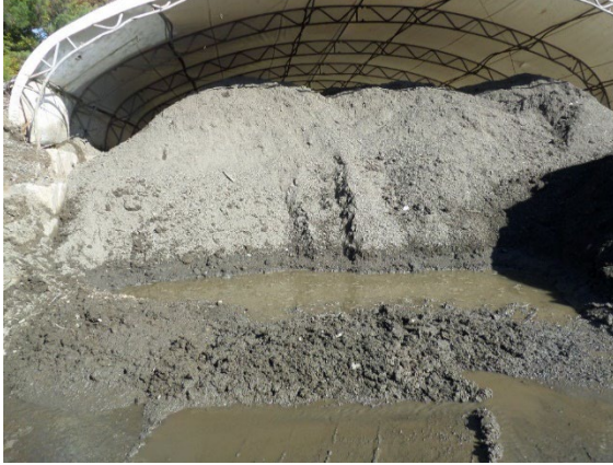
Figure 31: HTL. Bunkers. Observed stream of wastewater accumulated and comingled with ASR in right Bunker 11:19 am. View North.
