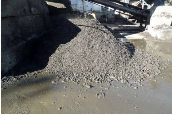
Figure 25: HTL. Adjacent Old Keebler Plant. Continue to generate New FVS heavies from back end during sampling Observed wastewater on ground. 10:37 am.
