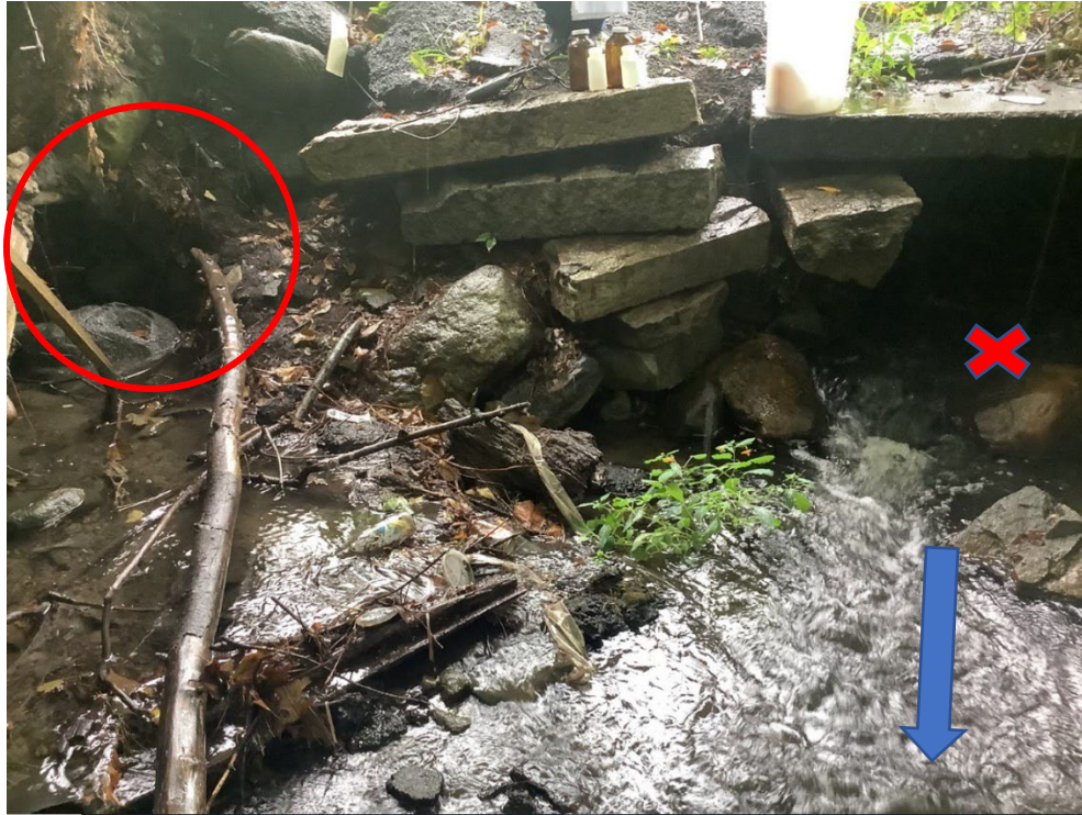
Brook: In-stream sample of Bloody Brook at the stream culvert on Brook St. Note “BrookOut” is located on the left side of the photo (red circle). Flow direction is indicated by a blue arrow. Sample point is indicated by a red “X”.
