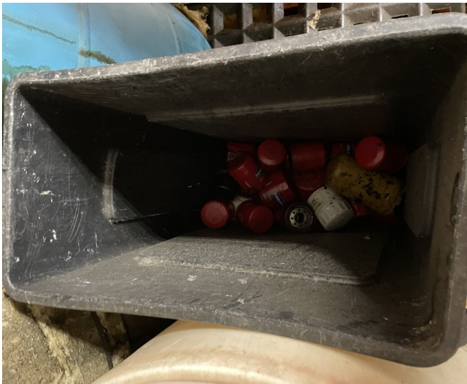
Picture 107 - UPR BUILDINGS & LAND DEPARTMENT- At the Fields and Roads Shop there was one (1) 20-gallon black container open on top with spent used oil filters impregnated with used oil not marked with the words, "Used Oil."
