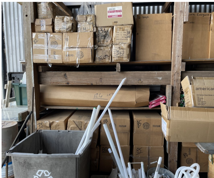
Picture 113 - UPR BUILDINGS & LAND DEPARTMENT- At the Universal Waste Storage Area there were sixty (60) square cardboard boxes (1'x1'x 4') packing over sixty (60) 4-foot spent fluorescent lamps, some open and not labeled with the words, "Universal Waste," or dated with their accumulation start dates.
