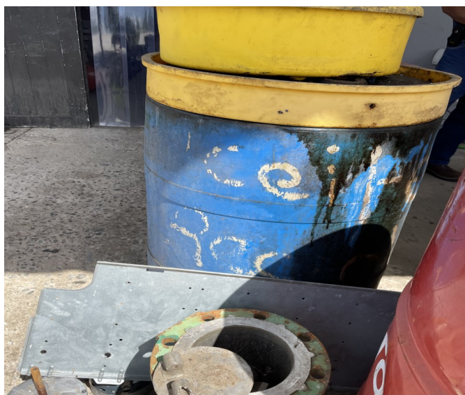
Picture 102 - UPR BUILDINGS & LAND DEPARTMENT- At the Refrigeration Shop, there was one (1) 55-gallon blue drum with a yellow drainage tray on top with used oil generated from draining compressors not marked with the words, "Used Oil"
