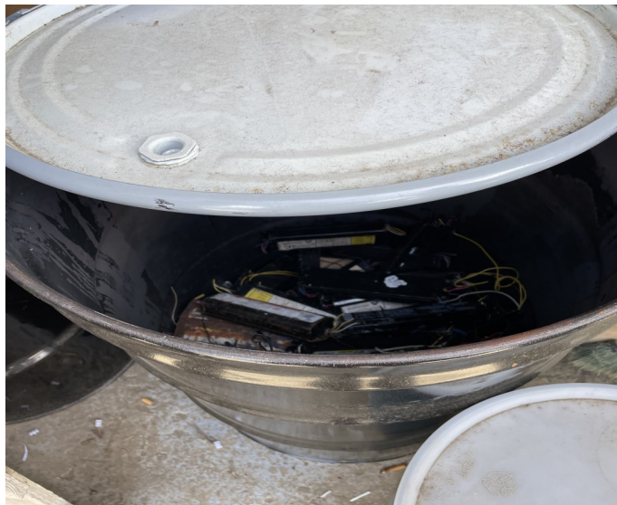
Picture 118 - UPR BUILDINGS & LAND DEPARTMENT- At the Universal Waste Storage Area there were two (2) 55-gallon black steel drums with lids containing "Ballast" which were removed from aluminum frames. None were clearly labeled with the words, "Universal Waste-Mercury Equipment," or dated.
