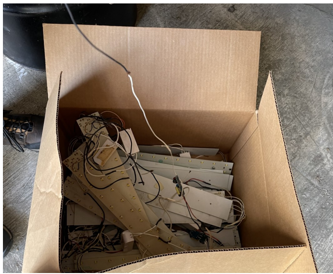
Picture 120 - BUILDINGS & LAND DEPARTMENT — At the Universal Waste Storage Area there was one (1) cardboard box (1'x1'x 2') open with LED light cards, and not labeled with the words, "Universal Waste-Mercury Containing Equipment," or dated.
