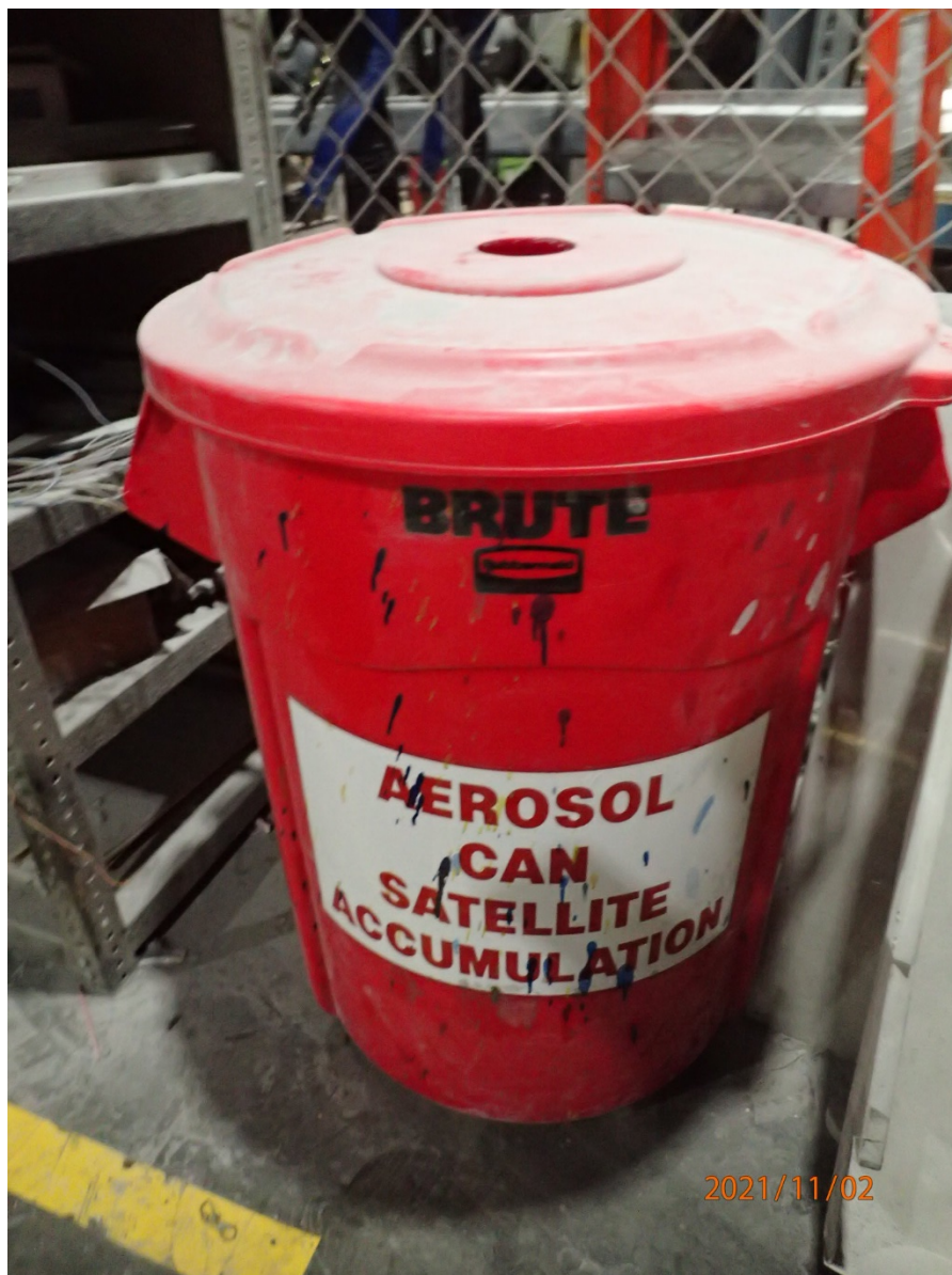
Photo 9: Spent aerosol cans were stored in a container which did not have a hazardous waste label or marked with an indication of hazard.
