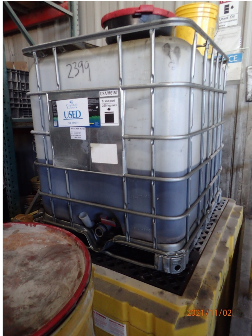
Photo 10: 250-gallon used oil tote.
