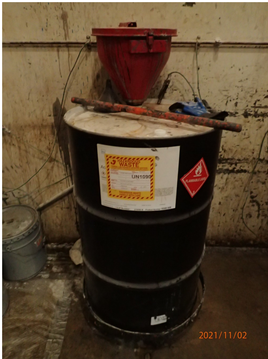
Photo 15: One (1) 55-gallon drum of spent solvents. The container was closed but was missing a hazardous waste label. This was corrected immediately onsite (Photo #15). The container was marked with an indication of hazard.
