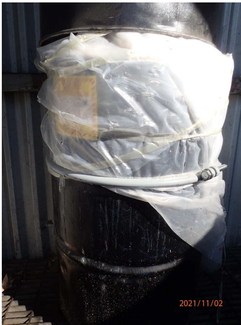
Photo 5: One (1) 55-gallon drum of waste acetone. The container was closed and labeled with the words “Hazardous Waste” and marked with an indication of hazard. The drum appeared to be bulging and the date was not clearly legible but appeared to be written as 05/ 2021. Mr. Shaver indicated the start accumulation date was over 90-days as well.
