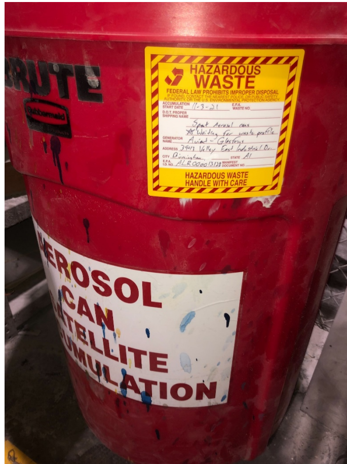
Photo 14: Photos of both containers of spent aerosol cans were submitted showing the containers labeled "Hazardous Waste".
