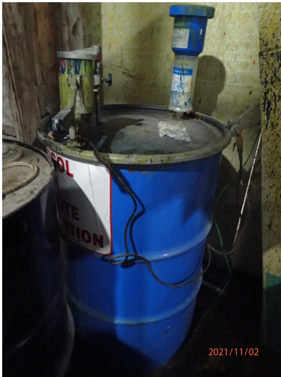
Photo 12: One (1) aerosol can puncture device attached to a waste container. The container was not labeled with the words hazardous waste or marked with an indication of hazard.
