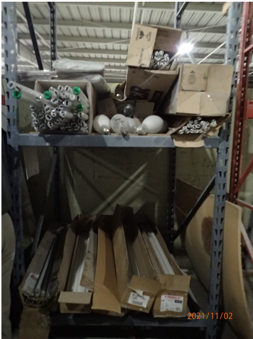
Photo 11: Eleven (11) boxes of Universal Waste (UW) fluorescent lamps. The boxes of UW were open, not labeled, and not dated.
