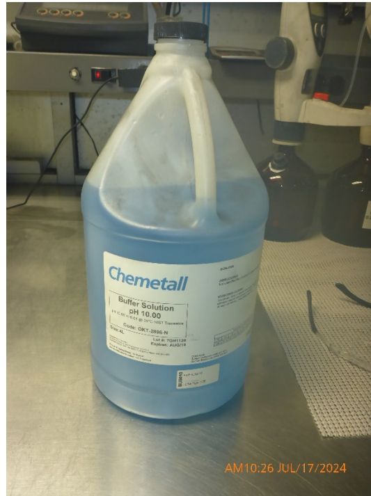
Photograph 5: Expired pH 10 buffer solution used for calibrating the pH meter.
