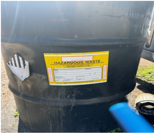
Photo-42 SAA Container with a DOT Class 9 Label
