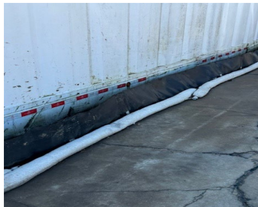
Photo-6 Spill Boom near Frac Tank
