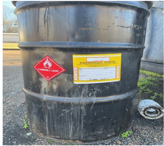
Photo-43 SAA Container with Flammable Label
