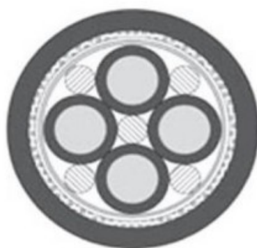
Figure 10: Representation of the complex internal structure of a CT cable
