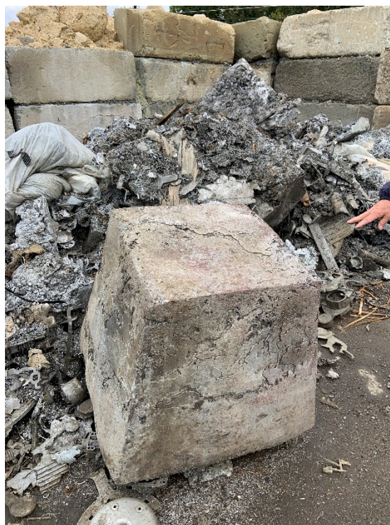
Figure 22: IMG_3091.jpg – Mr. Brown said this was an Aluminum Refractory Skull
