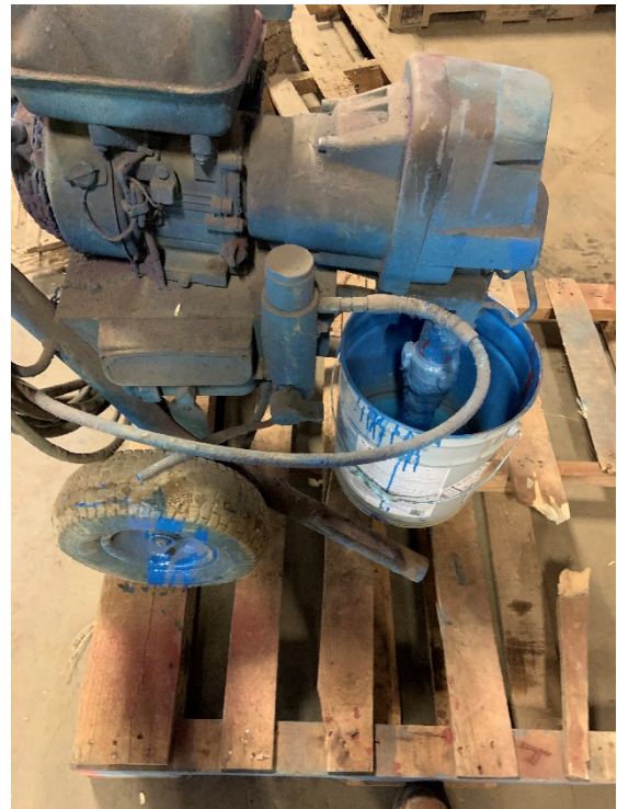
Figure 6: IMG_3075.jpg – Paint sprayer in the Fabrication Building
