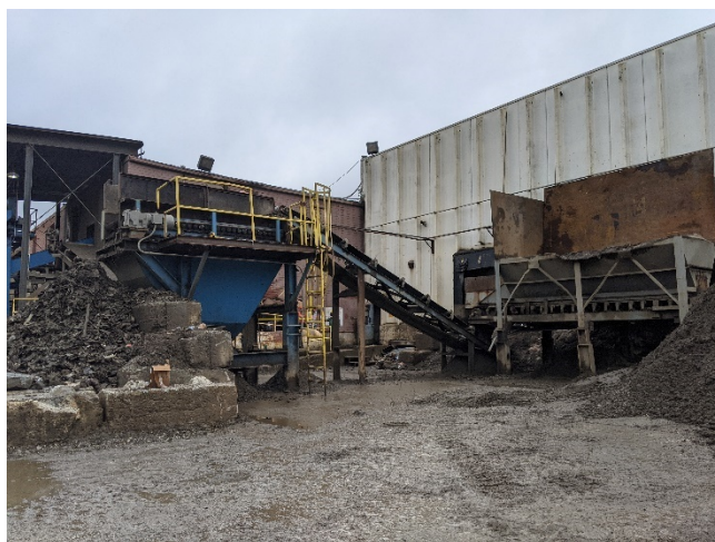
Figure 50: PXL_20211006_141553356.jpg – Initial Processing, sorting by particle size
