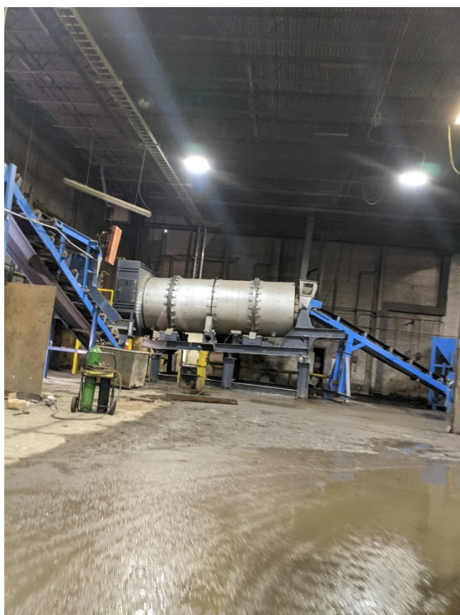
Figure 59: PXL_20211006_145257774.MP.jpg – Eddy Current Process used to recover Aluminum
