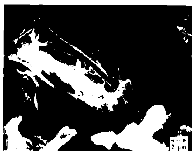
Fig. 1. Photomicrographs of particulate matter removed from thumbs and index fingers of laboratory workers. A. Aggregates from dry, unheated ring liner (initial magnification, \times 50 ). B. Aggregates from heated ring liner (initial magnification, \times 50 ). C. Particles of dry, unheated ring liner (initial magnification, \times 5,000 ). D. Particles of heated ring liner (initial magnification, \times 5,000 ).
