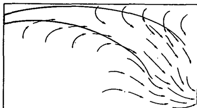
FIG. 6. ELEVATION VIEW OF IMPROPERLY LOCATED RETURN OUTLET
