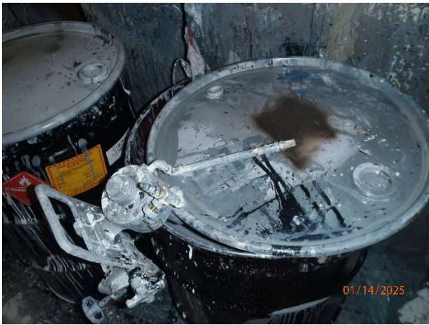
Picture 24 – Paint Area SAA container open
