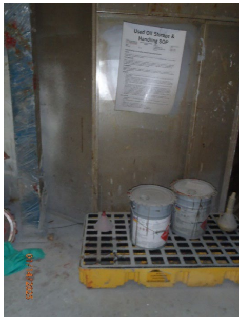
Picture 22 – Paint Area used oil container not closed or labeled
