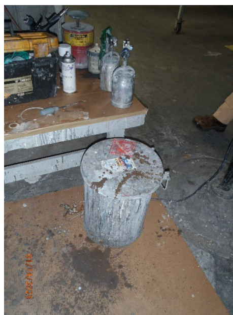
Picture 17 – Paint Area paint gun solvent rinse pot
