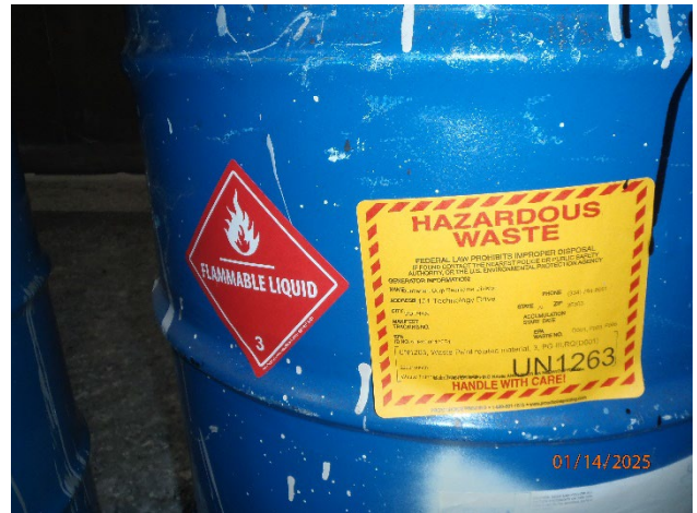
Picture 28 – Paint Area SAA container label
