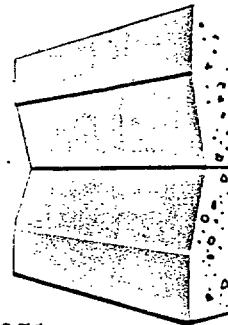
1951 Tapered Edges for Easier, Smoother Joint Finishing
