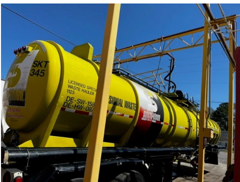
Photo #11 – Spent parts washer solvent storage tanker trailer.
