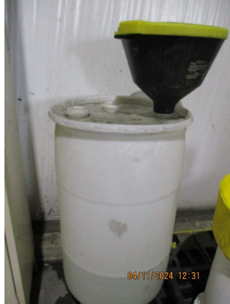
Photo 10: Raw Materials Warehouse CAA. 30-gallon container with no labeling at all.
