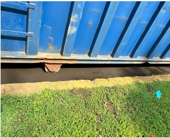
Photo-8 Used Oil puddling at a curb of a paved lot
