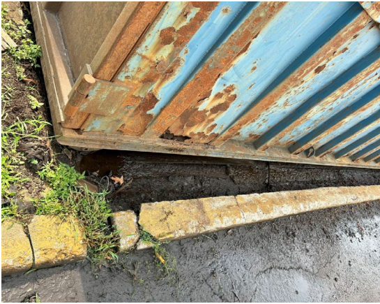
Photo-7 Used Oil leaking and puddling on ground from the sides of a rusted and deteriorated roll-off container
