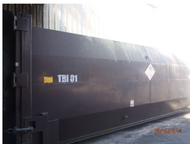
Picture 24 – Hazardous Waste Compactor
