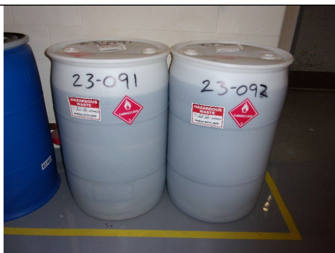
Figure 24: 10:11 AM Flammables Room Two of six 55-gallon containers with hazardous waste label, accumulation start date, and indication of the hazards of the contents.
