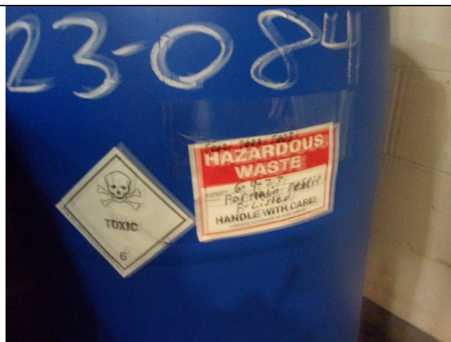
Figure 22: 10:08 AM Bulking/Blending Room (Photo 1 of 2) One 55-gallon container with hazardous waste label, accumulation start date, and indication of the hazards of the contents.
