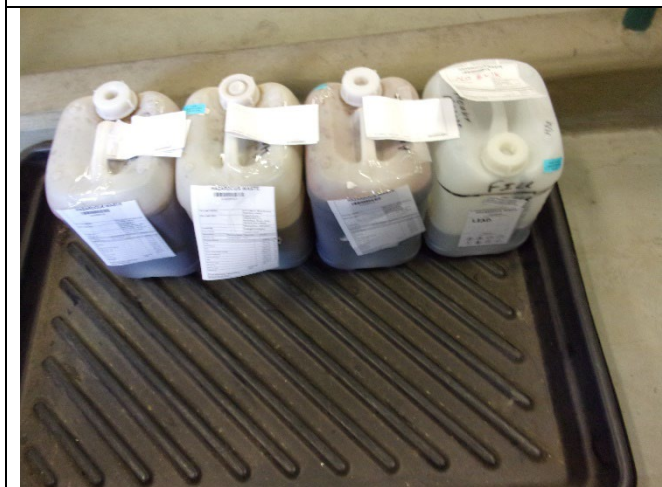
Figure 15: 9:57 AM Heavy Metal Section Four (4) 3-gallon containers with hazardous waste label, accumulation start date, and an indication of the hazards of the contents
