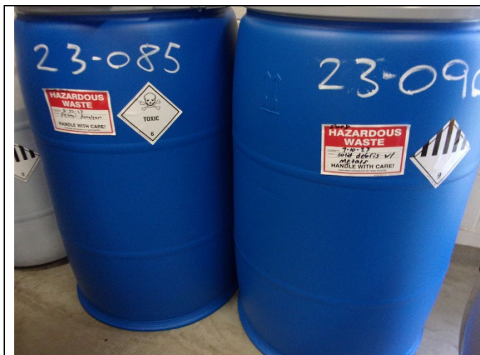
Figure 13: 9:52 AM Heavy Metal Section (Photo 1 of 2) Two (2) 55-gallon containers with hazardous waste label, accumulation start date, and indication of the hazards of the contents. One of the 55-gallon containers were not properly identified with an indication of the hazards of the contents.
