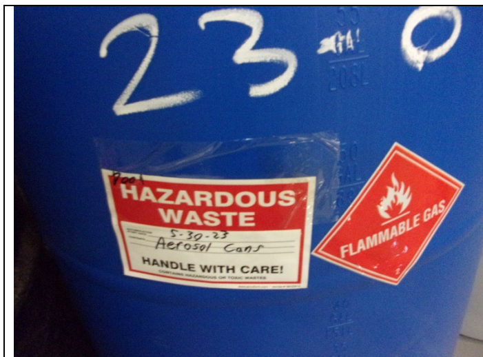
Figure 27: 10:12 AM Flammables Room Five of six 55-gallon containers with hazardous waste label, accumulation start date, and indication of the hazards of the contents.
