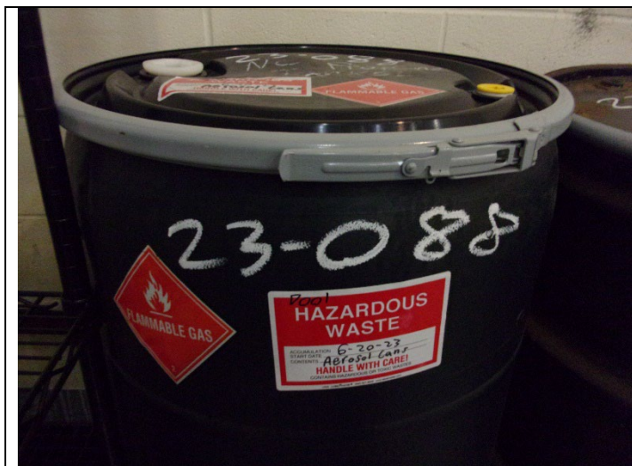
Figure 25: 10:12 AM Flammables Room Three of six 55-gallon containers with hazardous waste label, accumulation start date, and indication of the hazards of the contents.
