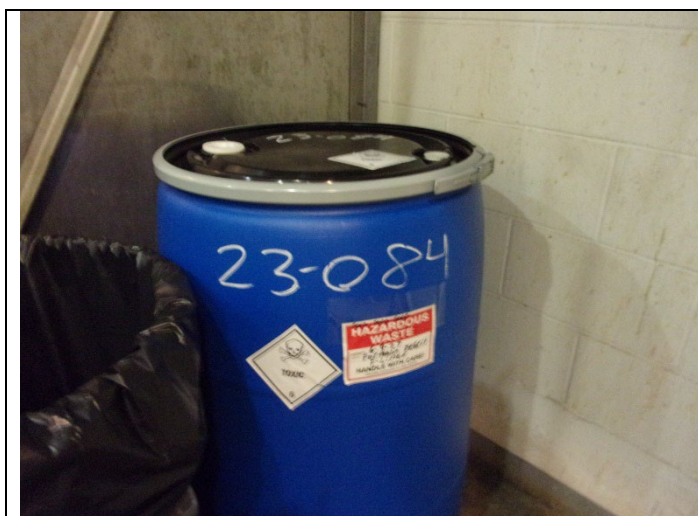
Figure 23: 10:09 AM Bulking/Blending Room (Photo 2 of 2) One 55-gallon container with hazardous waste label, accumulation start date, and indication of the hazards of the contents.
