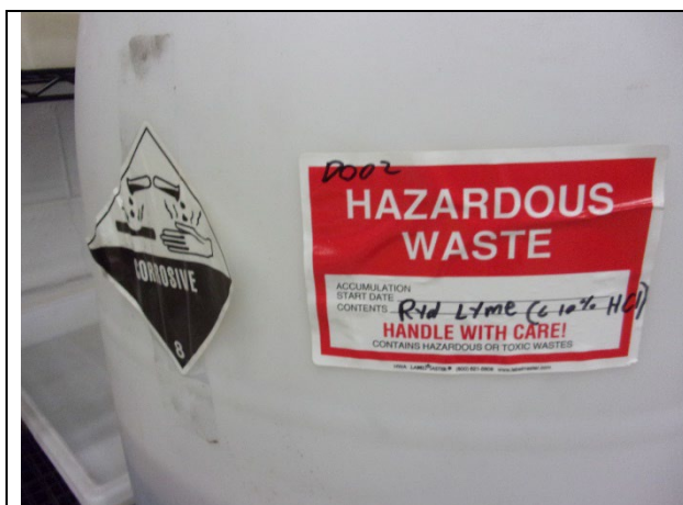
Figure 7: 9:43 AM Inorganic Acids Section (Photo 2 of 3) One 55-gallon container with hazardous waste label, accumulation start date, and indication of the hazards of the contents.
