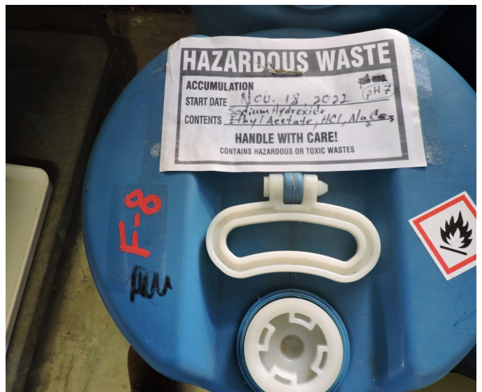
Picture 80 - UPR CENTRAL ACCUMULATION AREA— At the CAA, all drums were clearly labeled, coded as "D001", and identified with its hazard communication pictograms as, "Flammable Liquids."
