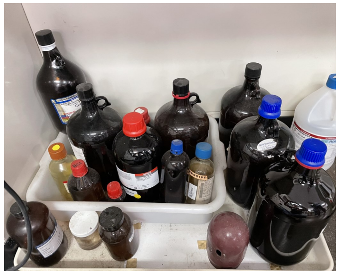
Picture 220 - UPR GENERAL ENGINEERING - At the Synthesis Laboratory, there were numerous “Unwanted Material,” including acetic, glacial, NaOH, FeCl 3 , cobalt with start accumulation date of August 31, 2018; and NaOH with start accumulation date of January 12, 2018. None dated,
