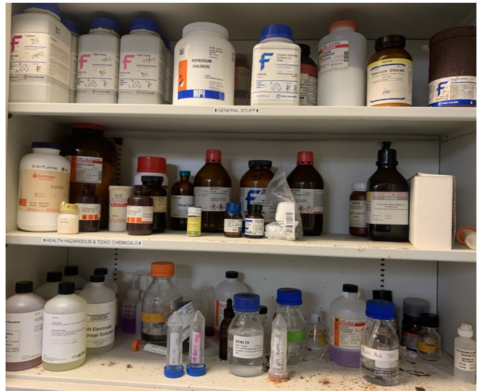
Picture 198 - UPR BIOLOGY DEPARTMENT At the Lab B-086, there were other chemical reagents stored in shelves without any physical means to protect each other from incompatibility of waste characteristics deteriorated, leaking, corroded, and spilling its content.
