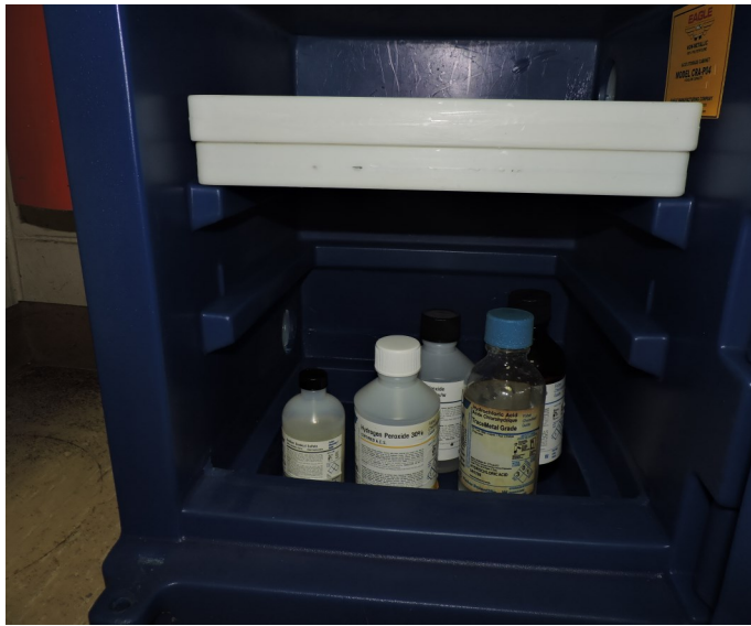
Picture 181 - UPR PHYSICS DEPARTMENT- At the Physics Labs, there were one (1) 1-L bottle phosphoric acid, and one (1) 1-L bottles hydrochloric acid, next to two (2) 1-L bottles of hydrogen peroxide and to one(1) 1-L bottle sodium dodecyl sulfate (explosive mixture in air) and not used since year 2004.
