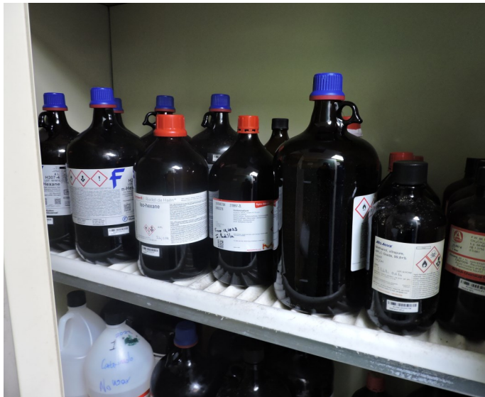
Picture 35 - UPR CIVIL ENGINEERING- At the Lab CI 018 Brown Cabinet Flammable there were six (6) 4-L ambar bottles containing Hexane, and n-Hexane, dated from 2005 – 2016.
