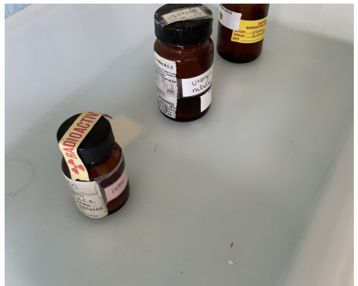
Picture 96- CENTRAL ACCUMULATION AREA — At the Hazmat Storage Building inside a plastic tray there were three (3) 50-ml (30-g) crystal containers with radioactive waste of "Uranyl Nitrate" and "Uranyl Acetate," stored for years without no hazardous waste determination or managed as hazardous waste.
