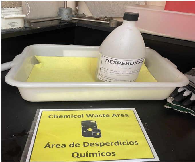
Picture 217 - UPR MECHANICAL ENGINEERING - At the Metallurgy Laboratory, there was one (1) 4-liter plastic bottle containing spent Nitric acid, Hydrochloric Acid, Ferric Chloride, Methanol, Ethanol from etching chemical analysis properly labeled as “Unwanted Materials,” and dated May 6, 2022.
