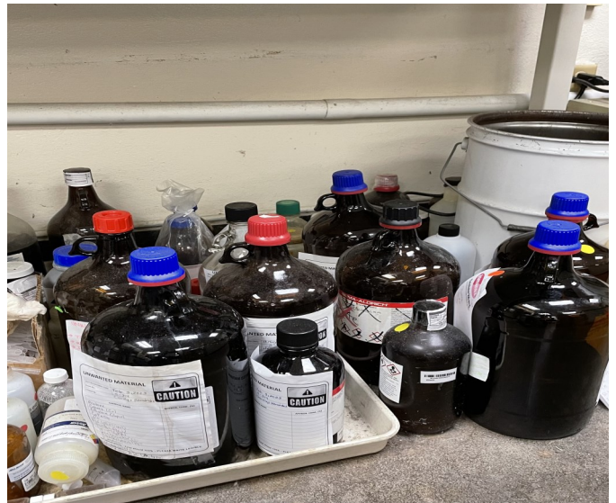
Picture 228 - UPR GENERAL ENGINEERING - At the Material Engineering and Characterization Lab, there were discarded, contaminated, unused chemical reagents, stored for a very long time (2008 in trays without any physical means to protect each other from incompatibility of waste characteristics).
