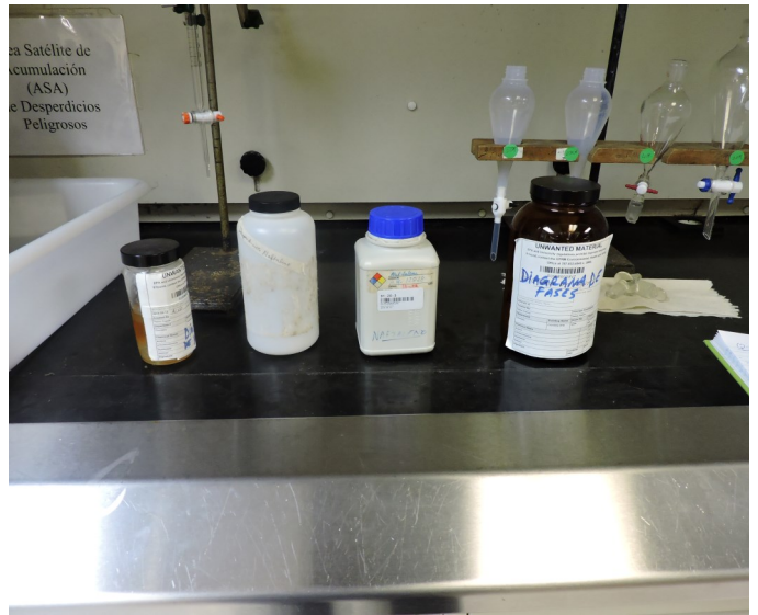
Picture 50 - UPR CHEMISTRY DEPARTMENT- At the Lab Q-050 there were two (2) 500-ml containers with a Napthalene Waste and one (1) 750-ml container with a Phase Diagram Waste no labeled as “Unwanted Material,” nor dated with its accumulation start date.
