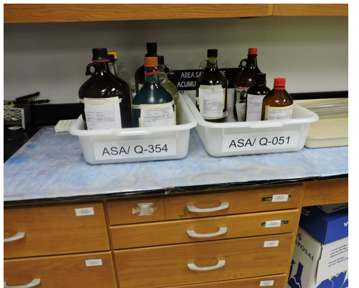
Picture 44 - UPR CHEMISTRY DEPARTMENT- At the Lab Q-051 SAA there were 10 bottles of “Unwanted Materials,” with spent chemical reagents generated at the laboratories properly labeled as “Unwanted Materials,” and dated with its accumulation start date but not segregated by compatible characteristics
