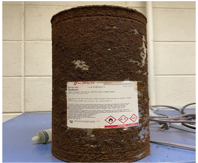
Picture 166 - UPR PHYSICS DEPARTMENT- At the Physics Lab F-123, the bottles of acid, flammable and reactive solvents were stored together with an abandoned sodium metallic bar. All seemed very old, very dry, unstable; had leaking metal lids, moisture, labels vanished, and violent reaction, and explosion.
