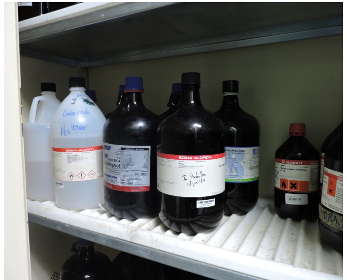
Picture 36 - UPR CIVIL ENGINEERING— At the CI 018 Brown Cabinet Flammable there were Eight (8) 4-L plastics and ambar bottles containing Methanol, Water HPLC Grade, Ehtyl Acetate, and Xylene, dated from 2005 – 2014. The Ethyl Acetate was labeled as “Non in Use Contaminated.”
