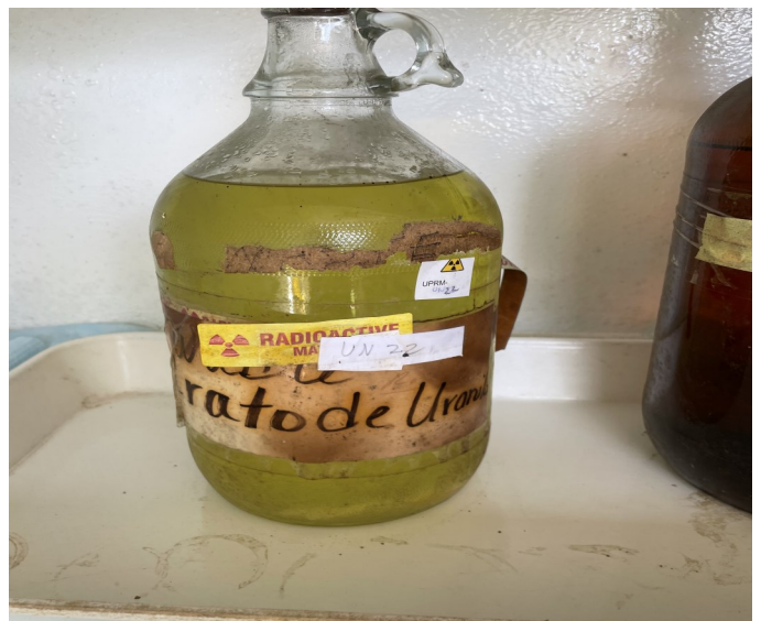
Picture 212 - UPR AGRICULTURAL DEPARTMENT - At the Nematology Laboratory, there three (3) 1-gallon crystal containers with radioactive waste of "Uranyl Nitrate" and/or "Uranyl Acetate," stored for years without no hazardous waste determination nor managed as hazardous waste due to corrosivity.
