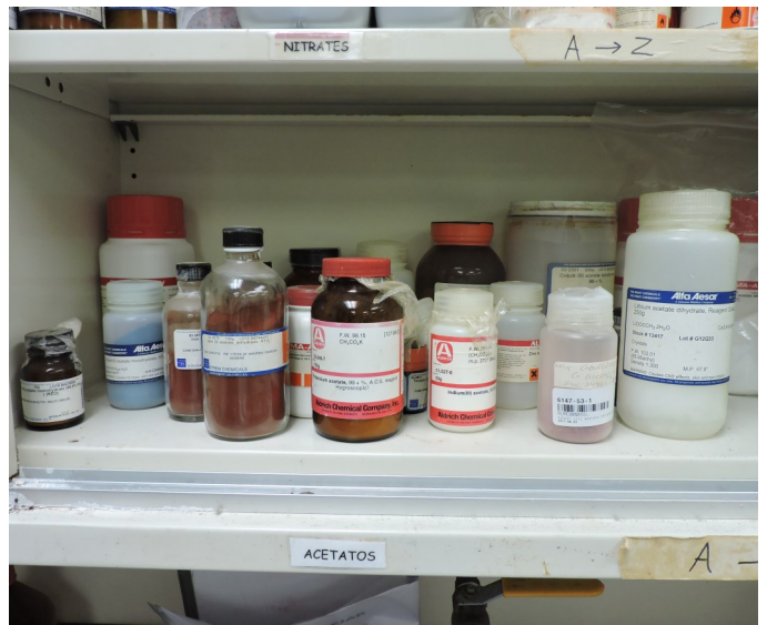
Picture 158 - UPR PHYSICS DEPARTMENT- At the Physics Lab F-129, there was potassium Acetate stored next to Iron Acetate “moisture sensitive” possible incompatible chemical reagents stored together without mean of any physical segregation. Iron Acetate is air sensitive and should be stored under inert gas..
