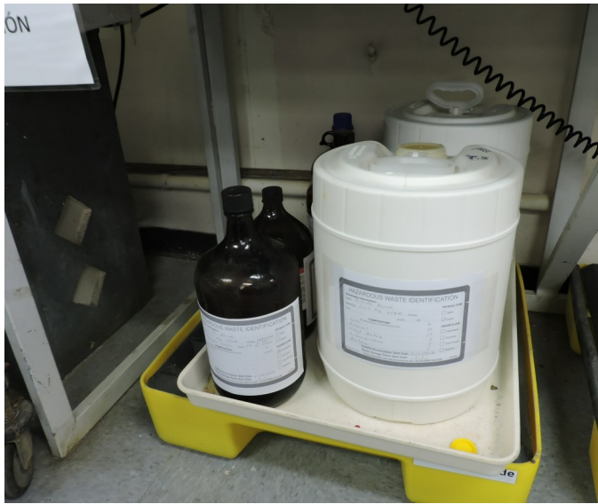
Picture 21 - UPR CIVIL ENGINEERING- At the Lab CI 018 there were two (2) 5-gallon white containers with Methanol, Ethyl Acetate, Dichloromethane and Acetone both labelled as “Hazardous and dated with its accumulation start date of March 1, 2023, but not labeled as “Unwanted Materials.”
