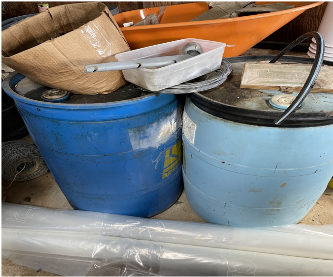
Picture 129 - UPR ALZAMORA FARM- At the Mechanic Shop, there were two (2) 55-gallon blue plastic drums, with spent de-greaser not labeled with their waste content. No hazardous waste determination has been made on the contents of the two 55-gallon drums at the Mechanic Shop.
