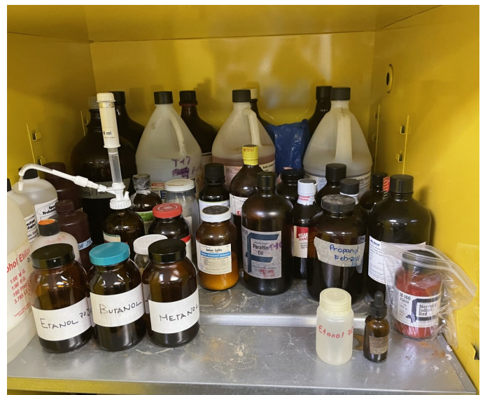
Picture 188 - UPR BIOLOGY DEPARTMENT - At the Lab B-026 there was a yellow cabinet identified as "Flammable" with methanol, butanol, ethanol, propanol, ethyl alcohol, sodium sulfite, paraffin oil, mercuric iodine red and buffer solution non compatible (i.e., Acetic Acid Glacial, Ethanol, Sodium Sulfite).
