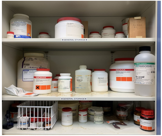
Picture 202 - UPR BIOLOGY DEPARTMENT At the Lab B-086, there were some chemical reagents were stored for a very long time (i.e., over a year or more January 14, 2009) in shelves without any physical means to protect each other from incompatibility of waste characteristics (Explosive vs. Corrosive).
