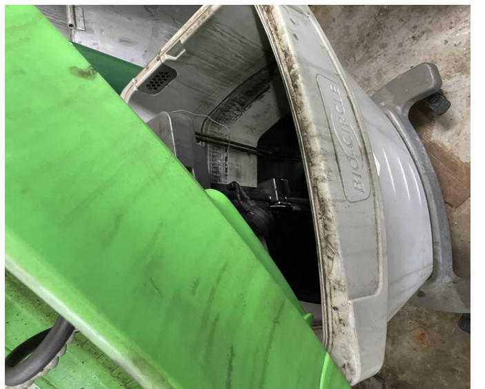
Picture 100 - UPR BUILDINGS & LAND DEPARTMENT- At the Mechanic Shop there was one (1) part-washer tray-container machine which uses CB-100 degreaser (e.g., biodegradable water-based cleaner and degreaser) to clean up auto parts, but diesel was used as a degreaser in the part-washer machine.
