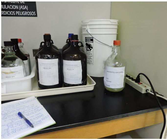
Picture 53 - UPR CHEMISTRY DEPARTMENT- At the Lab Q-046 SAA there were numerous containers with discarded or spent chemical reagents generated at the laboratories most of them properly labeled as “Unwanted Materials,” but properly dated with their accumulation start dates .
