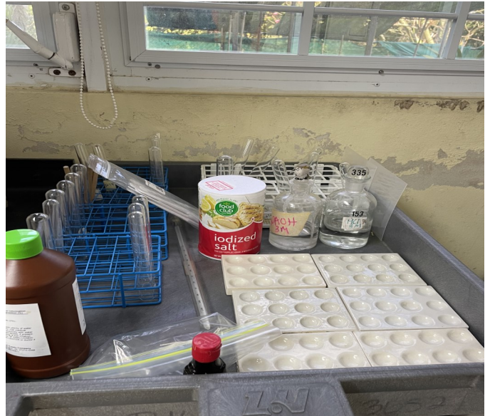
Picture 186 - UPR BIOLOGY DEPARTMENT - At the Lab B-020 there was on a testing table, EPA Inspector observed iodized salt, NAOH liquid solution, and HCl stored next to each other.
