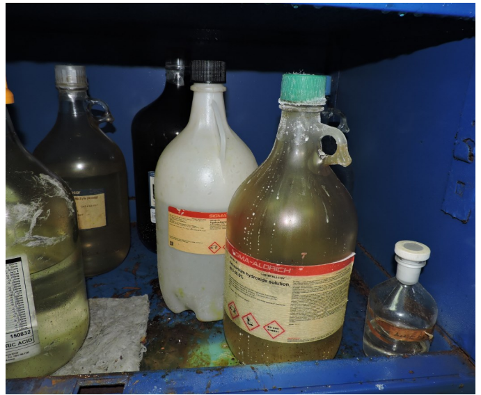
Picture 170 - UPR PHYSICS DEPARTMENT- At the Physics Lab F-123, there was one (1) 4-L ambar bottle Ammonium Hydroxide stored in the cabinet may read violently with strong acids such as hydrochloric, sulfuric, and nitric, dimethyl sulfate, halogens and an abandoned sodium metallic bar since year 2004.
