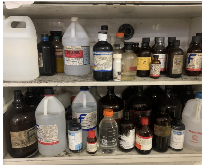
Picture 196 - UPR BIOLOGY DEPARTMENT - At the Lab B-073, there were chemical reagents were deteriorated with vanished labels, corroded, spilling its content and stored for a very long time.
