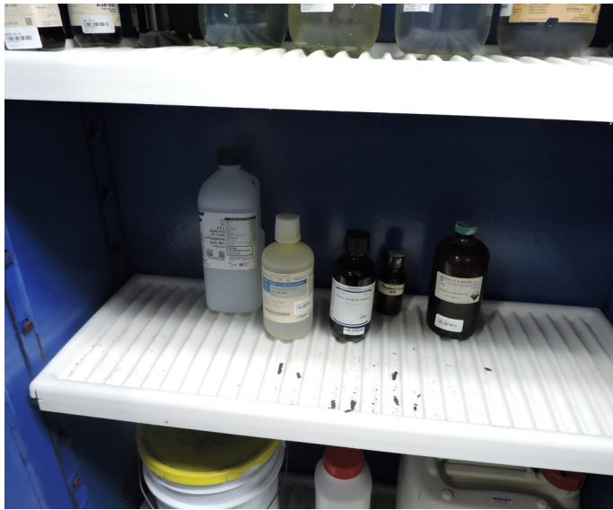
Picture 33 - UPR CIVIL ENGINEERING- At the Lab CI 018 Blue Cabinet Corrosive there were two (2) 2.5-L and ½-L plastic and ambar bottles containing Phosphoric Acid, dated 2014, some old and in deteriorated conditions, not in use and abandoned .
