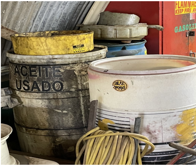
Picture 109 - UPR BUILDINGS & LAND DEPARTMENT- At the Fields and Roads Shop there was one (1) 55-gallon white drum with a yellow drainage tray on top with used oil generated from draining landscape equipment marked with the words, "Aceite Usado."
