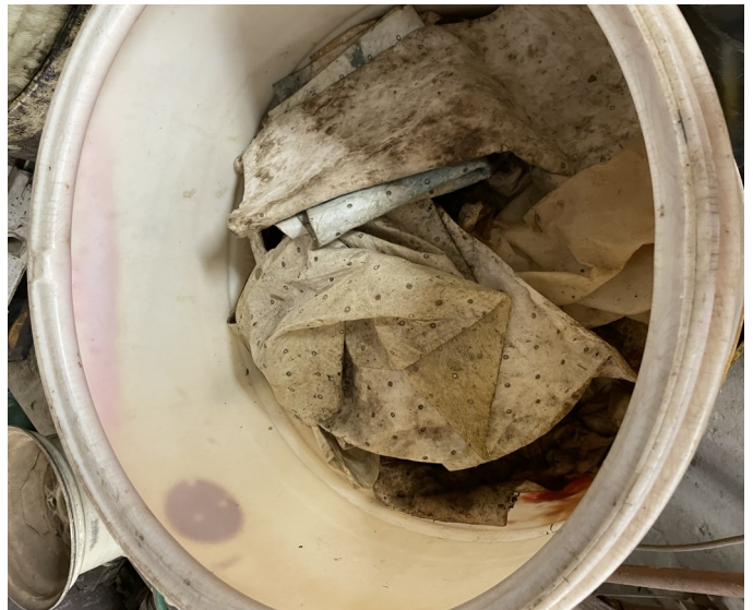
Picture 110 - UPR BUILDINGS & LAND DEPARTMENT- At the Fields and Roads Shop there was one (1) 55-gallon white drum with rags impregnated with used oil not marked with the words, "Used Oil."
