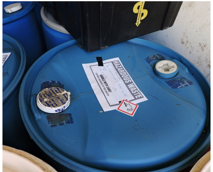
Picture 92 - CENTRAL ACCUMULATION AREA — At the Hazmat Storage Building there were nine (9) 55-gallon blue/white drums containing Chiller Washing Water – D002), clearly labeled with the words, “Hazardous Waste,” and all dated with their accumulation start dates of January 12, 2023 and hazard pictograms.
