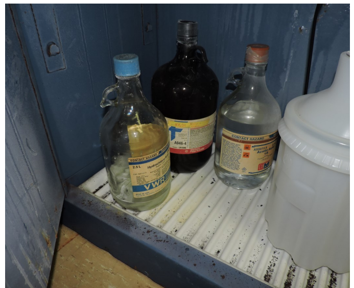
Picture 184 - UPR PHYSICS DEPARTMENT - At the Physics Labs, there were two (2) 4-L bottle with hydrochloric acid, next to a one (1) 4-L with acetic acid , next of one (1) 4-L bottle of ammonium hydroxide, next to one (1) bottle of acetone not stored in a compatible manner and not used since year 2004.
