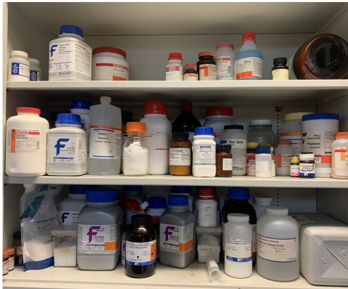
Picture 197 - UPR BIOLOGY DEPARTMENT At the Lab B-086, there were some chemical reagents were stored for a very long time (i.e., over a year or more October 20, 2015) in shelves without any physical means to protect each other from incompatibility of waste characteristics.
