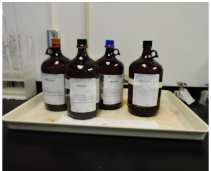
Picture 52 - UPR CHEMISTRY DEPARTMENT— At the Lab Q-050 (SAA No. 2) on top of a laboratory cabinet table there were four (4) 4-liter amber containers with a spent Unknown Waste, all labeled as “Unwanted Material,” but properly dated with their accumulation start dates.
