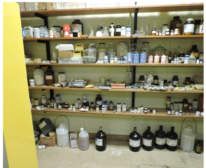
Picture 180 - UPR PHYSICS DEPARTMENT - At the Physics Laboratory, Inspectors observed numerous expired chemical, discarded, contaminated, various unused chemical reagents, deteriorated and stored for a very long time (2004) in shelves without any protection, or incompatibility of waste characteristics
