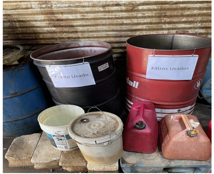
Picture 126 - UPR ALZAMORA FARM- At the Mechanic Shop there was one (1) 55-gallon red drum open on top with spent used oil filters impregnated with used oil not marked with the words, "Used Oil," (Spanish "Filtros Usados").
