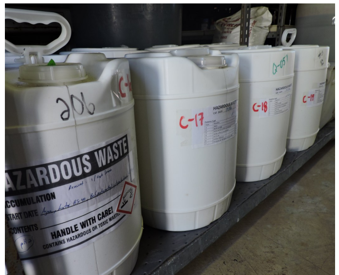
Picture 84 - UPR CENTRAL ACCUMULATION AREA— At the CAA, there were Six (6) 5-gallon white drums containing corrosive liquid wastes (Sodium Hydroxide, Hydrochloric Acid, Sulfuric Acid-D002), clearly labeled with the words, “Hazardous Waste,” and dated with their accumulation start dates.
