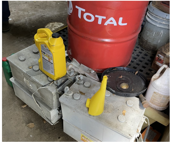
Picture 130 - UPR ALZAMORA FARM- At the Mechanic Shop there were five (5) vehicle and truck batteries on the floor discarded without control showing evidence of leakage, and damage that releases of Sulfuric Acid, and not labeled with the words, "Hazardous Wastes," nor dated.
