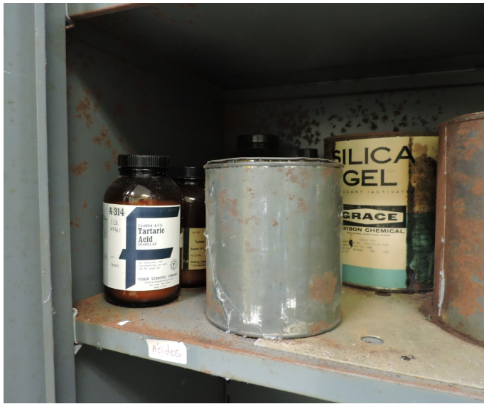
Picture 161 - UPR PHYSICS DEPARTMENT- At the Physics Lab F-129, inside the gray solids' cabinet, there were unknown chemical reagents stored next to acids (i.e., tartaric acid, some seemed abandoned, not in use or stored in lieu of being disposed of as a hazardous.
