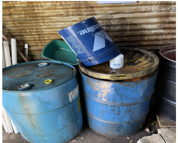
Picture 128 - UPR ALZAMORA FARM- At the Mechanic Shop there were two (2) 55-gallon blue plastic drums with used oil not marked with the words, "Used Oil."
