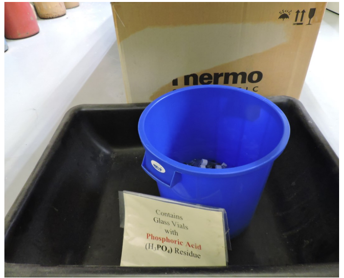
Picture 154 - UPR PHYSICS DEPARTMENT- At the Geology Lab F-107 there was one (1) 4-gallon bucket with a spent vials containing Phosphoric Acid (100%) no labeled as “Unwanted Material” nor dated with its accumulation start date.
