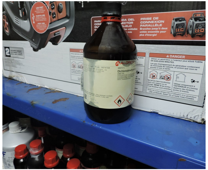
Picture 26 - UPR CIVIL ENGINEERING- At the Lab CI 018 Blue Cabinet Flammable there were two (2) 4-L bottles containing Dichloroethane leaking and covered with moisture, dated January 22, 2011 which decomposes into carbon dioxide and in present of heat it can produce toxic fumes such methylene chloride.
