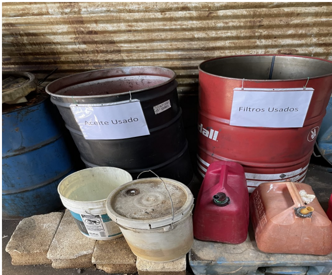
Picture 127 - UPR ALZAMORA FARM- At the Mechanic Shop there was one (1) one (1) 55-gallon black steel drum open with used oil not marked with the words, "Used Oil."
