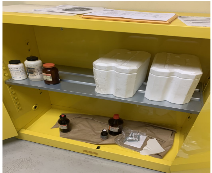
Picture 204 - UPR BIOLOGY DEPARTMENT- At the Lab B-086, EPA Inspectors also observed that the cabinet stored some explosive chemical reagents such as ammonium hydroxide and nitric acids, and not “Flammable.”
