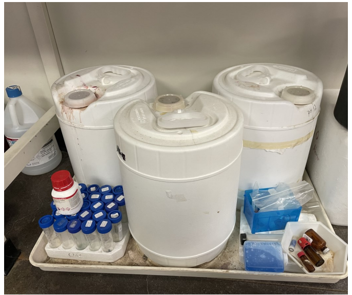
Picture 226 - UPR GENERAL ENGINEERING - At the Material Engineering and Characterization Lab, there was SAA with discarded hazardous wastes unlabeled, not dated, or managed under the LMP, which included three (3) 5-gallon white containers with corrosive wastes (pH>12.5) stored next organic wastes.
