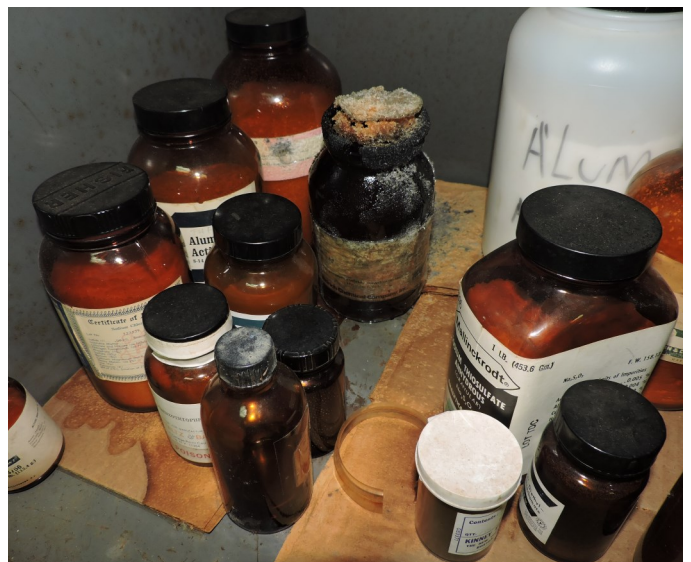
Picture 164- UPR PHYSICS DEPARTMENT— At the Physics Lab F-129, there was Hydrofluoric acid, broken, and leaking acid on cabinet shelf stored next to Sodium bromide, Sodium thiosulfate (violently reacts with strong oxidizers, and acids) and Silica gel incompatible with HF, stored together possible
