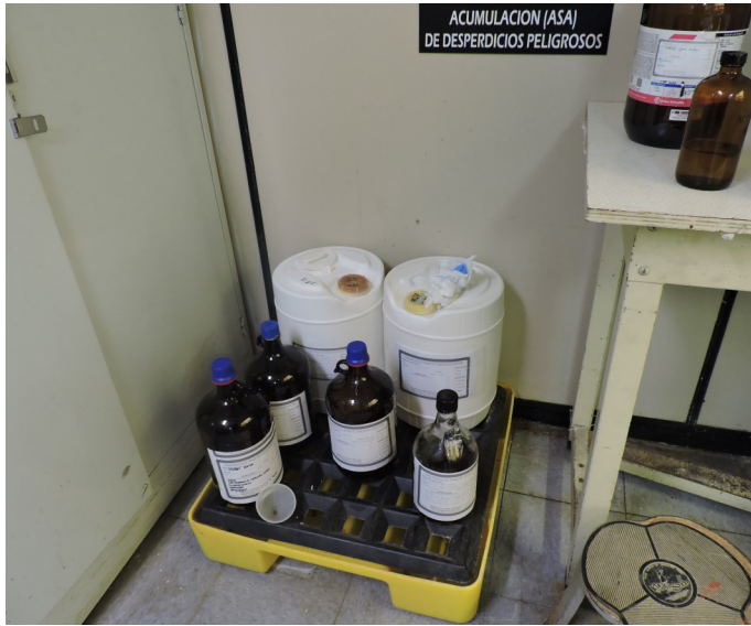
Picture 25 - UPR CIVIL ENGINEERING- At the Lab CI 018 SSA-1 there were two (2) 5-gallon white containers with organic wastes both labeled as “Hazardous Waste,” and dated with its accumulation start date nor labeled as “Unwanted Materials.”
