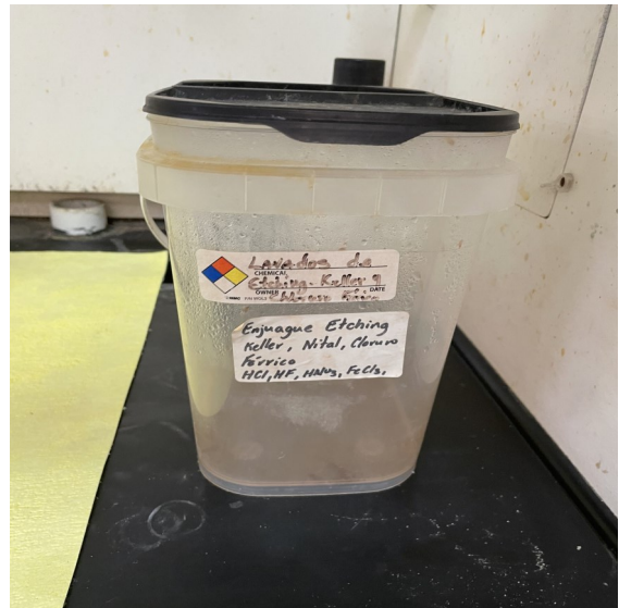
Picture 216 - UPR MECHANICAL ENGINEERING - At the Metallurgy Teaching Laboratory, inside an extractor fume hood there was one (1) 2.5-gallon plastic container with spent etching solution from washing metal etching testing containing solution wastes of HCl, HF, FeCl 3 , and HNO 3
