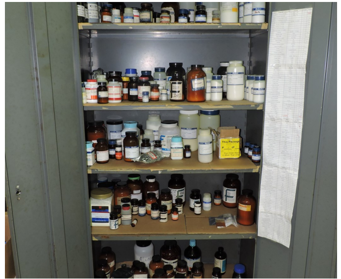
Picture 178 - UPR PHYSICS DEPARTMENT- At the Physics Lab F-458, there were sodium sulfite, activated carbon, flourene, yttrium nitrate stored next of potassium dichromate, and strontium hydroxide, strontium acetate, lanthanum chloride in an incompatible manner at risk of fire or explosion.
