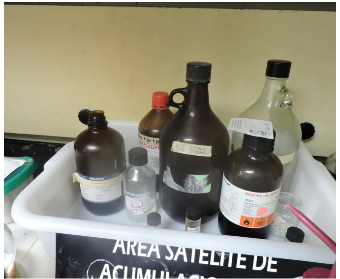
Picture 70 - UPR CHEMISTRY DEPARTMENT- At the Lab Q-159 inside an extractor hood there were numerous (approximately over ten 10) “Unwanted Materials,” containing discarded or spent chemical reagents generated at the laboratories not labeled as “Unwanted Materials,” open and not dated.
