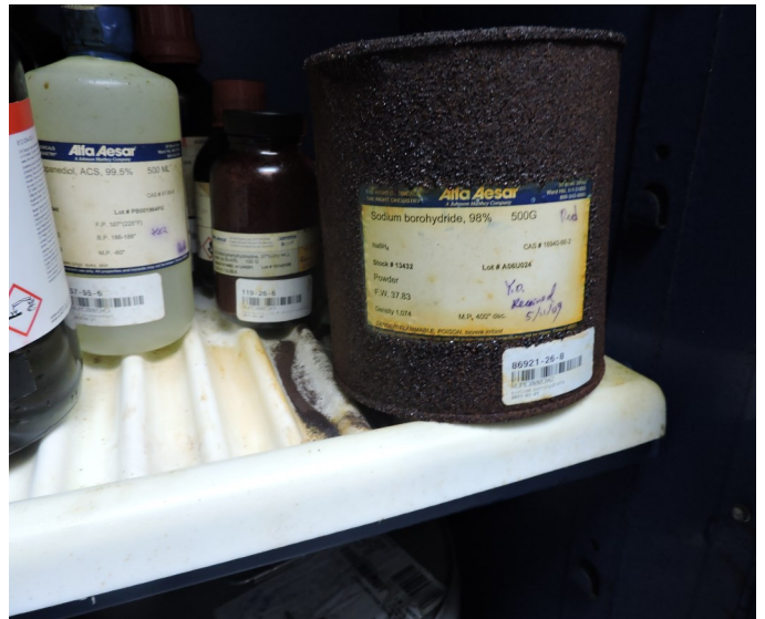
Picture 28 - UPR CIVIL ENGINEERING— At the Lab CI 018 Blue Cabinet Flammable there was one (1) 1-gallon metal can with Sodium Borohydride, dated January 01, 2011, leaking on the tray, fully corroded, covered with water moisture and seemed decomposed forming sodium hydroxide and hydrogen.
