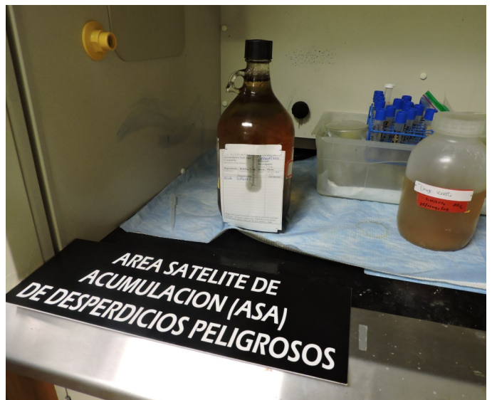
Picture 68 - UPR CHEMISTRY DEPARTMENT - At the Lab Q-165 there was one (1) 1-gallon ambar container with a spent Sulfuric Acid waste labeled as “Unwanted Materials,” leaking, and dated with its accumulation start date of September 28, 2021, which exceeded over six months of the LMP collection protocols.
