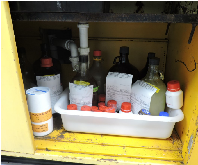
Picture 49 - UPR CHEMISTRY DEPARTMENT- At the Lab Q-050 at the Satellite Accumulation Area under a laboratory cabinet there were numerous bottles containing discarded or spent chemical reagents generated at the laboratories not labeled as “Unwanted Materials,” nor properly dated.
