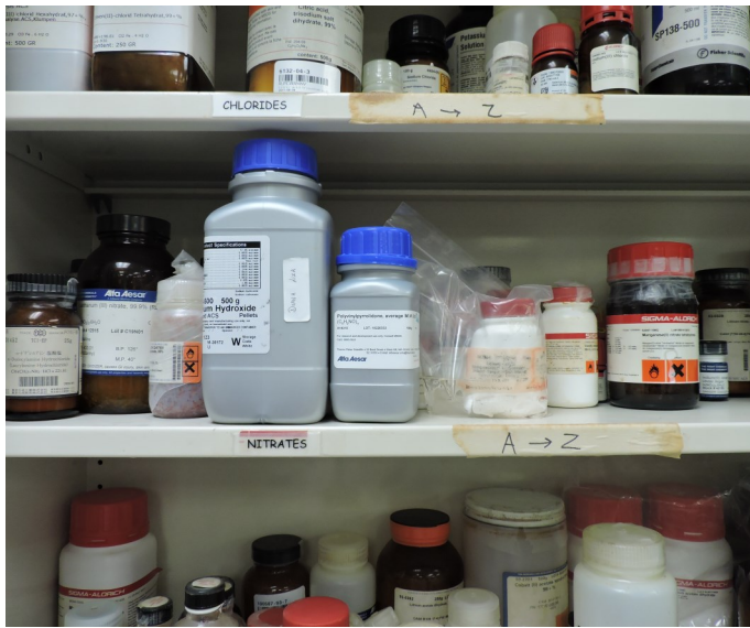
Picture 157 - UPR PHYSICS DEPARTMENT- At the Physics Lab F-129, there was sodium hydroxide stored next to Polyvinylpyrrolidone; possible incompatible chemical reagents stored together without mean of physical segregation nor hazardous waste determination.
