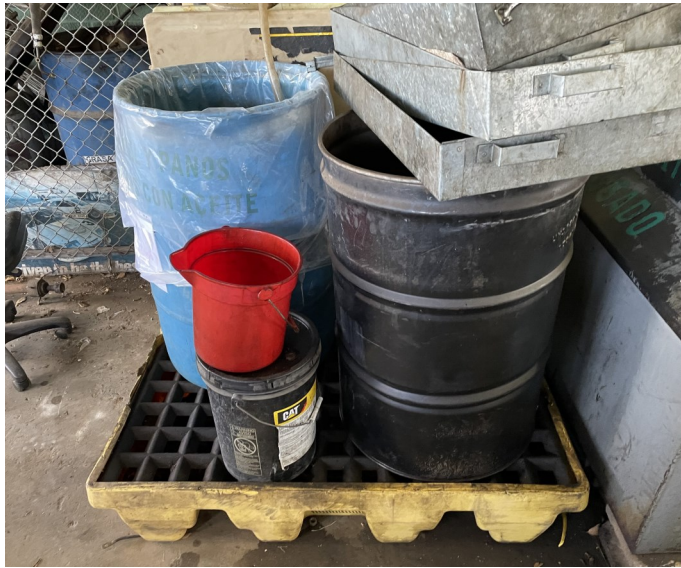
Picture 101 - UPR BUILDINGS & LAND DEPARTMENT- At the Mechanic Shop, there was one (1) 55-gallon black drum open on top with spent used oil filters impregnated with used oil not marked with the words , "Used Oil."
