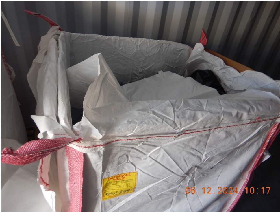
View of paint debris tote stored with top opened with no accumulation start date inside the CAA {Photograph 18, Attachment 1}
