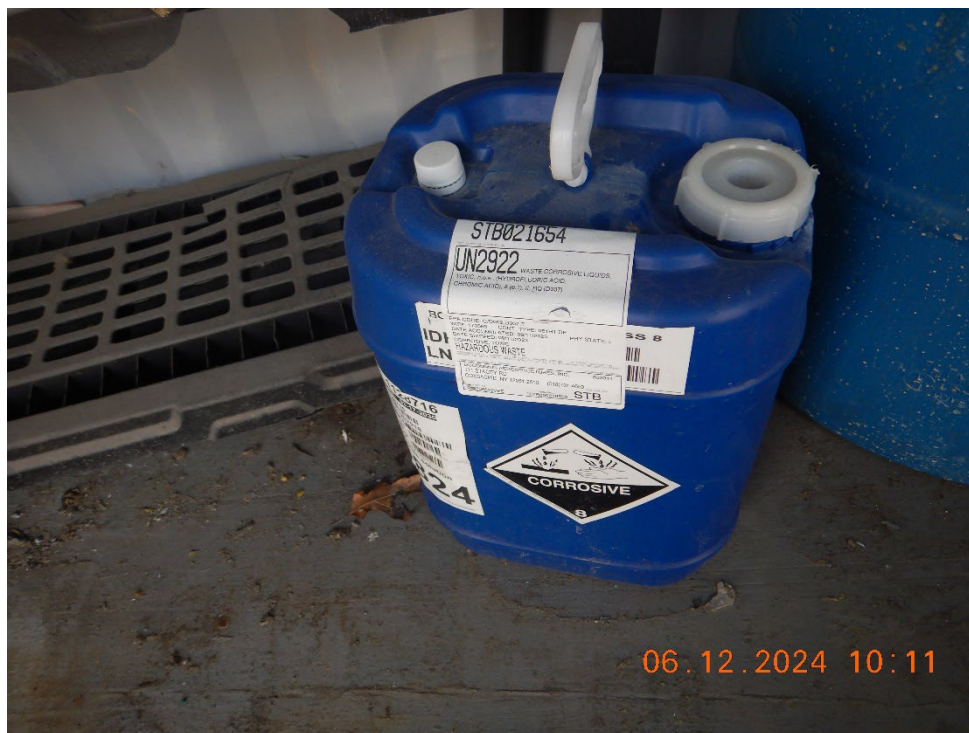
View of 5-gallon carboy containing hazardous corrosive waste stored past the 90-day storage period inside bay 1 of CAA. {Photograph 12, Attachment 1}
