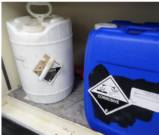
Formulated. QA Laboratory. Fume hood cabinet near laboratory entrance. Observed a white 5-gallon container marked with the words "spent chromic acid". The container was not marked/labeled with the words hazardous waste. The facility emailed a photograph to FDEP and EPA on April 16, 2021, showing the container marked/labeled with the words hazardous waste. Photograph 3 taken at 11:31 a.m.
