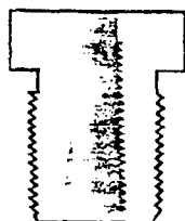
Figure 2.5 Standard Fusible Plug for Ton Containers
