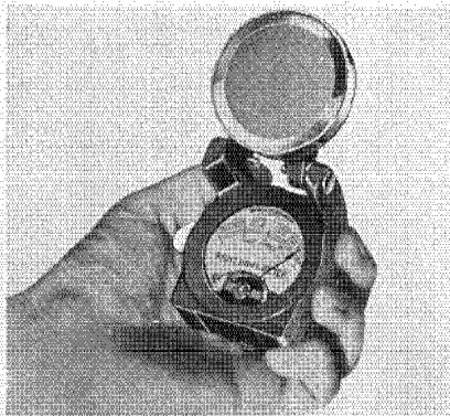
This ingenious device, used for making illumination surveys, measures light intensity in various parts of the plant
