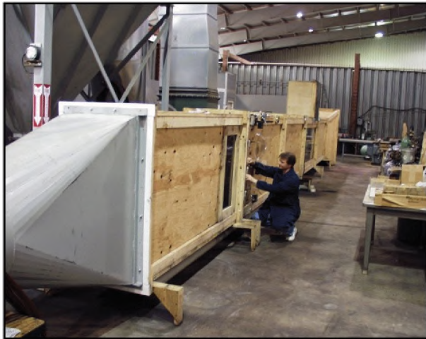
Wind tunnel used to evaluate shield dust entrainment.
