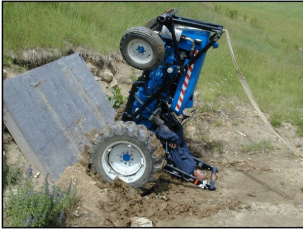
Rear upset test with mannequin.
