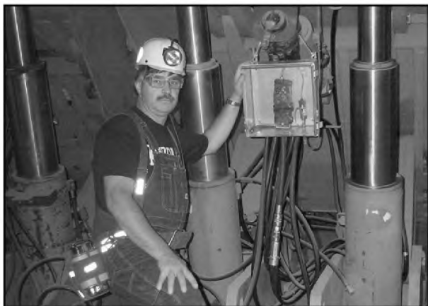
A researcher checks a continuous recording methanometer installed on longwall shields at critical locations on the active face during long-term emission studies.
