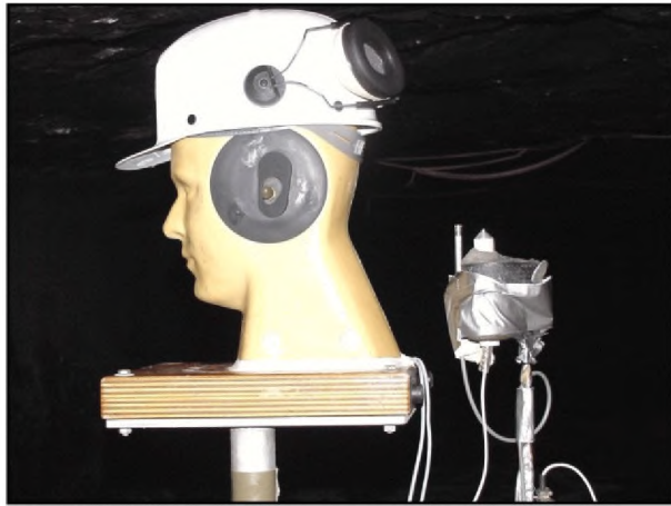
Measurement of pressure wave in the Lake Lynn underground mine.
