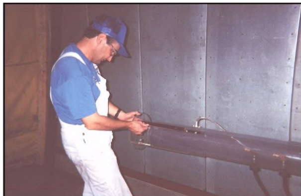
Water-powered scrubber testing to improve air movement and dust capture.
